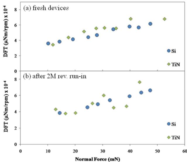
Fig. 5: (a) DFT values for bare Si and TiN coated systems. Both systems follow the linear relationship between DFT and normal load. (b) DFT values for raceways after 2M revolutions of run-in. Si raceways remain consistent, while the TiN coated systems begin to exhibit erratic behavior.
