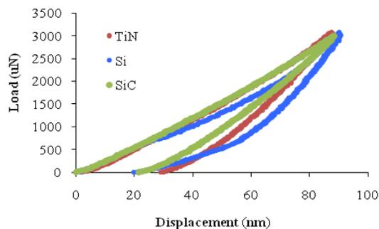
Fig. 2: Characteristic load/displacement curves obtained for Si, SiC and TiN
