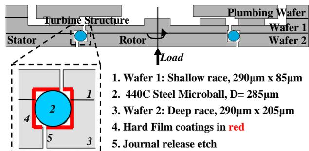
Fig. 1: Cross section schematic of the microturbine tribology test device with a close-up of the raceway.
