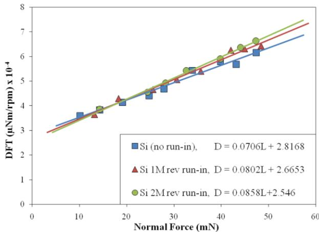
Fig. 3: DFT relationship from 10mN-50mN normal load in a silicon raceway/steel ball microturbine system.
