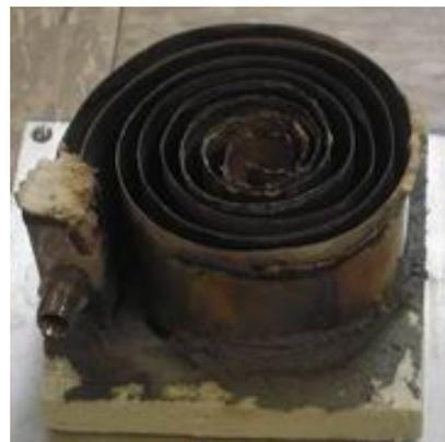
Fig. 1: An open-top Swiss roll heat-recirculating burner.
