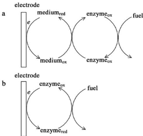
**Fig. 3.** Types of electron transfer pathway. (a) Mediated electron transfer (MET). (b) Directed electron transfer (DET).
