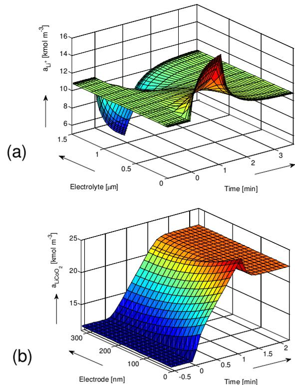
**Fig.7.** Development of concentration profiles during (a) 51.2 C discharge in the solid-state electrolyte and (b) in the  $\text{LiCoO}_2$  electrode.
