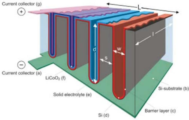
**Fig. 8.** Geometric definitions of 3D trenches.
