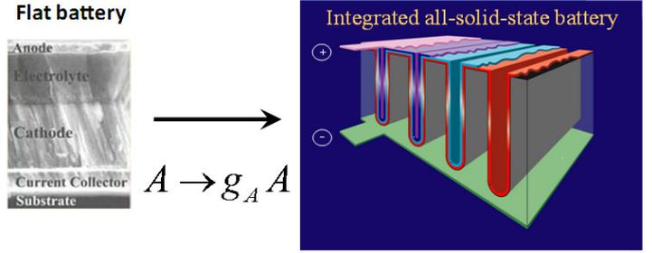
**Fig. 9.** The concept of geometrical area gain.
