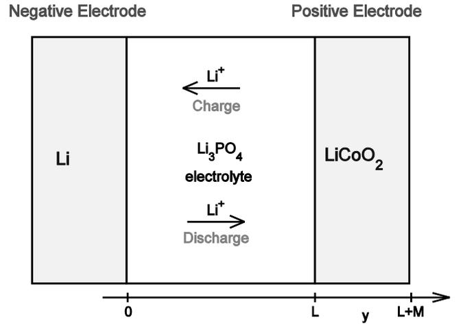
**Fig.4.** Schematic representation of a planar all-solid-state Li-ion battery.
