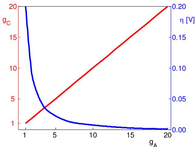
**Fig. 11.** Relation between relative capacity increase (red line/scale) and overpotential (blue line/scale) as function of geometrical area gain (current is kept constant in the simulations).
