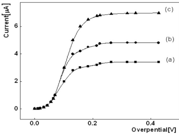
**Fig. 5.** Simulation of current-voltage curves of the anode of a BFC in a buffered electrolyte (PBS pH 7.2) containing 1 mM Ferrocene as mediator. (a) Ferrocene+Gox +1 mM Glucose; (b) Ferrocene+Gox +10 mM Glucose; (c) Ferrocene+Gox +20 mM Glucose.
