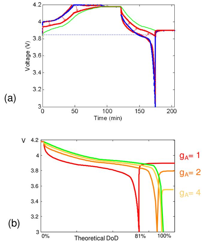
**Fig. 10.** Reduction of the overpotentials of the flat Li-ion battery resulting from 3D-structuring (a) and improvements in the kinetics as function of the surface area enlargement (b).
