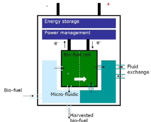
**Fig. 1.** Block scheme of an autonomous energy supply unit, consisting of a bio-fuel cell, a power management and a 3D-micro battery.
