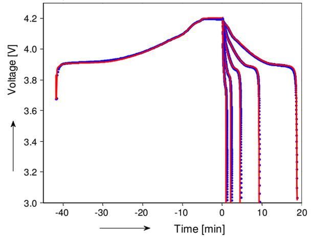
**Fig. 6.** Voltage profiles of an solid-state Li-ion battery during charge and discharges with various C-rates.
