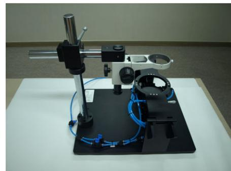
Fig. 4: The custom-made mask aligner
