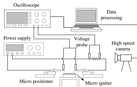
Figure 8. Experimental setup
