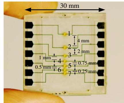
Figure 7. Fabricated micro-igniter
