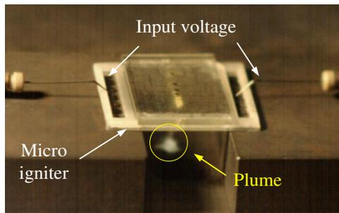
Figure 9. Firing test of micro-igniter
