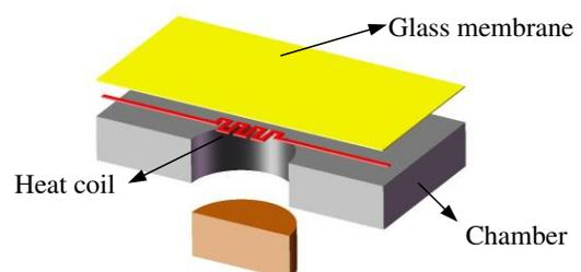
Figure 1. Schematic of micro-igniter
