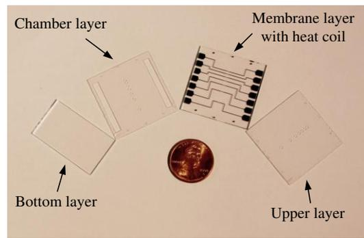
Figure 6. Fabricated layers of micro-igniter
