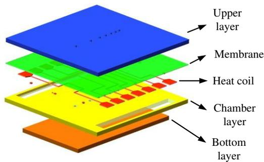
Figure 2. Designed micro-igniter for firing test
