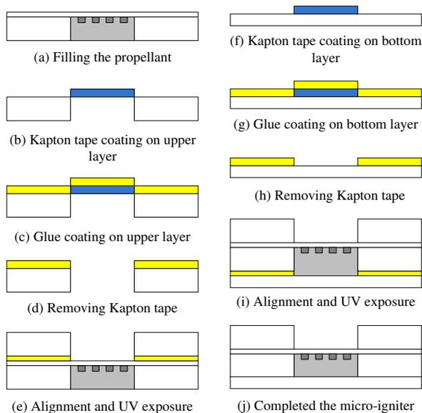
Figure 5. Final integration process of micro-igniter
