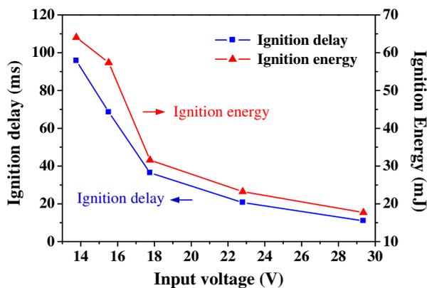
Figure 10. Ignition delay and energy as a function of voltage
