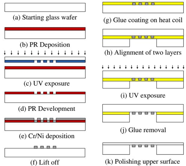
Figure 3. Fabrication process of membrane layer and integration process of membrane and chamber layers
