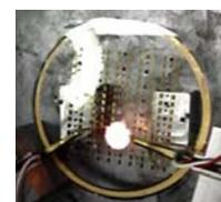
Fig. 13: Propellant combustion after its ignition by the nanothermite.
