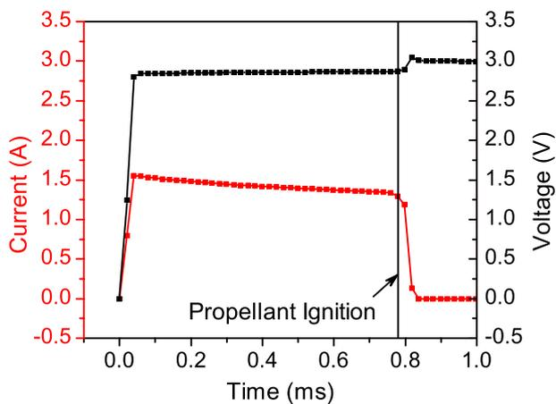
Figure 5: Representative current and voltage traces for a 2000 nm thick aluminum igniter (input power = 4.1 W).
