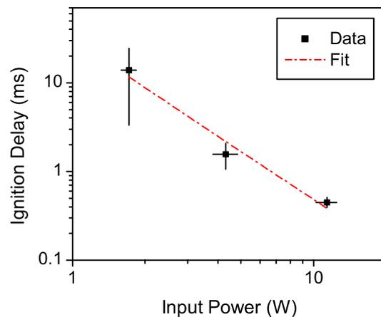
Figure 4: Ignition delay time vs. input power for the 2000 nm thick igniters. Each data point represents the mean of 4 separate trials.
