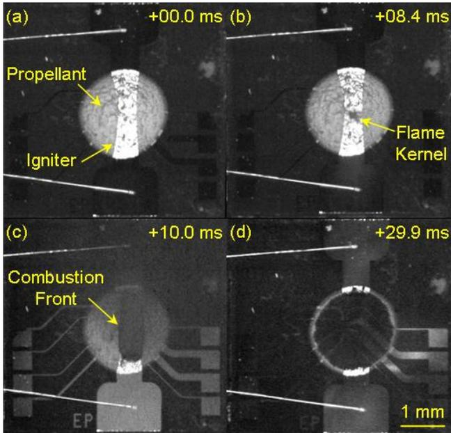
Figure 2: High-speed video frames of a 2000 nm thick aluminum igniter undergoing Joule-heating ignition (mean input power = 1.7 W): (a) before ignition, (b) appearance of flame kernel, (c) flame spreading and peeling of igniter, and (d) post combustion. Time stamp is given relative to start of voltage pulse.
