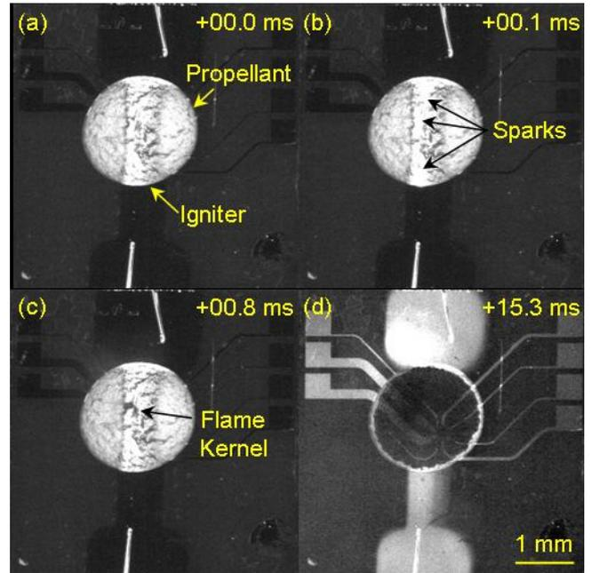
Figure 3: High-speed video frames of a 500 nm thick silver igniter undergoing spark-induced ignition (mean input power ~ 30 W): (a) before ignition, (b) appearance of sparks, (c) flame kernel formation, and (d) post combustion. Time stamp is given relative to start of voltage pulse.
