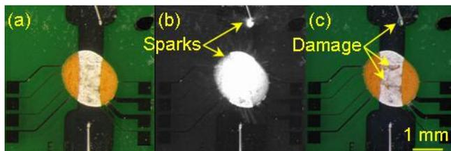
Figure 7: Micrographs of a 500 nm thick aluminum igniter that failed to ignite due to spark-induced igniter damage: (a) before, (b) during and (c) after voltage pulse.
