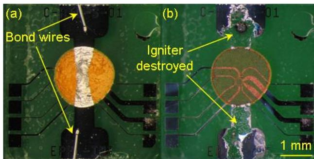
Figure 6: Before and after micrographs of a 500 nm thick aluminum igniter that was destroyed by voltage pulse.
