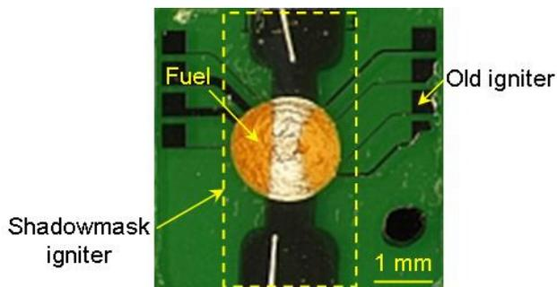
Figure 1: Dark field micrograph of a 500 nm thick, E-beam evaporated, aluminum igniter deposited on glass substrates using a rotary-planetary substrate holder. The shadow mask igniter is the vertical dog-bone shape running overtop the orange fuel drop. The contact pads lining the sides of the chips and interconnects leading underneath the fuel drops are the igniters from [7] and are unrelated to the present study (indicated as “old igniter”).
