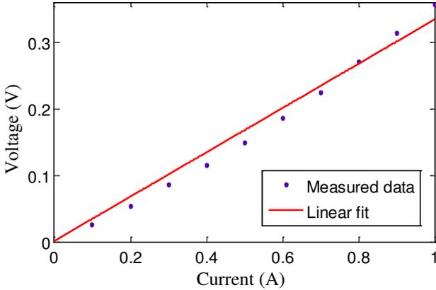
Fig. 5: Open-circuit voltage vs. input current amplitude at 103 Hz excitation.
