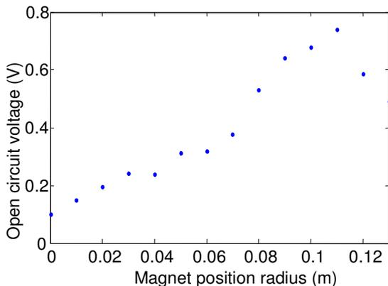
Fig. 6: Open-circuit voltage amplitude vs. magnet position for 1 A current at 103 Hz.
