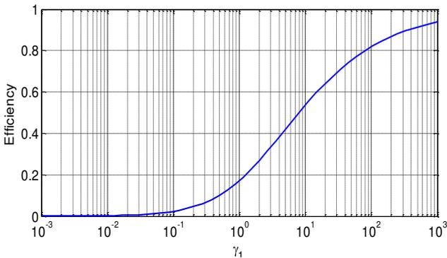
Fig. 8: Maximum efficiency vs. transmitting coupling strength, when  $\gamma_2 \gg 1$  and  $\gamma_1 \ll \gamma_2$ .
