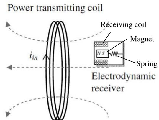
Fig. 1: Schematic of the proposed WPT system.
