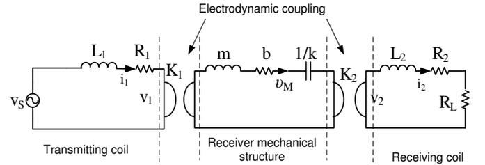
Fig. 7: Equivalent circuit model of the electro-dynamically coupled WPT system.
