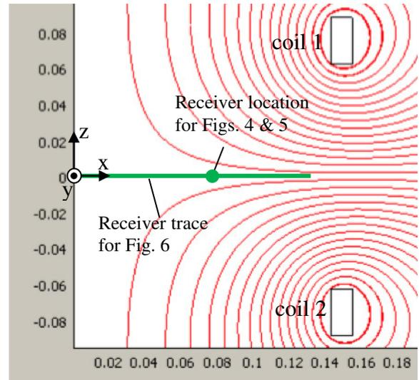
Fig. 3: Streamline plot of the flux density generated by the counter-directional coil currents using 2D axisymmetric FEM simulation on COMSOL Multiphysics.
