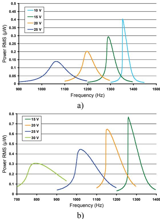
Fig. 6: AC RMS power output for different bias voltages. Load resistance:  $820 \text{ k}\Omega$ . a) Excitation amplitude:  $20 \text{ m/s}^2$ , b) Excitation amplitude:  $40 \text{ m/s}^2$ .
