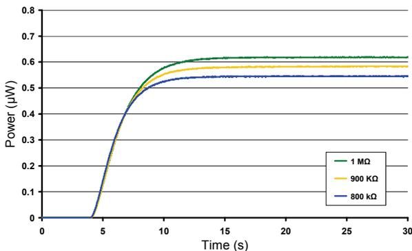
Fig. 10: Charging response of the energy storage capacitor (2 µF) at different load resistances. Bias voltage: 15 V, Excitation amplitude: 30 m/s<sup>2</sup>.
