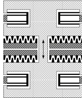
Fig. 1: Schematic view of the transducer structure incorporating triangular electrodes.
