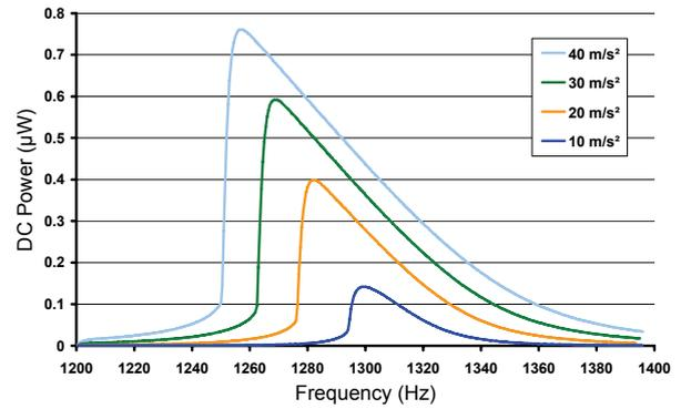
Fig. 7: DC power output for different excitation amplitudes. Bias voltage:  $15 \text{ V}$ , Load:  $800 \text{ k}\Omega$
