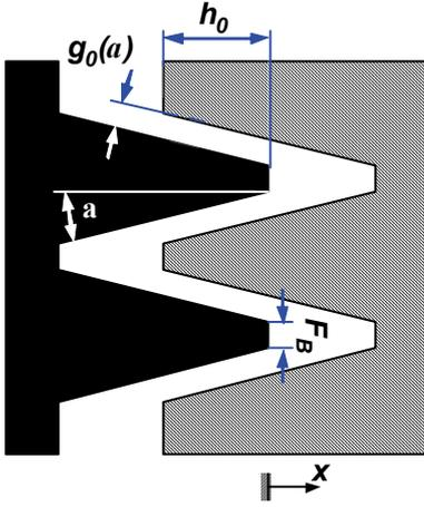
Fig. 2: Schematic view of the electrode geometry.
