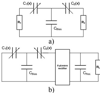
Fig. 3: Electrical context: a) symmetric circuit with two load resistors; b) circuit with full-bridge rectifier, energy storage capacitor and load resistor.
