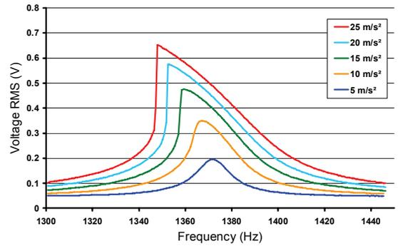
Fig. 4: AC RMS voltage for different excitation amplitudes. Bias voltage: 10 V, Load: 820 k $\Omega$
