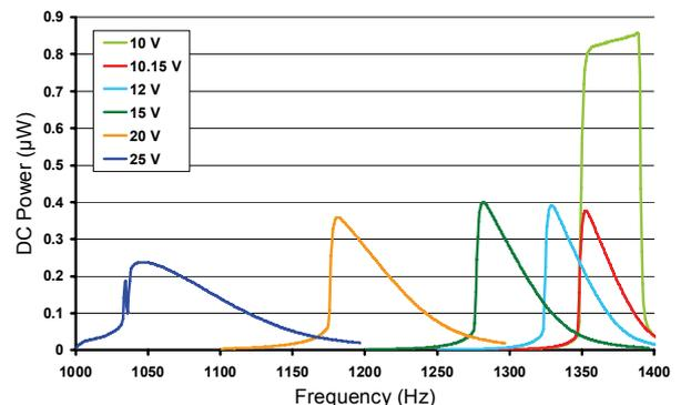
Fig. 8: DC power output for different bias voltages. Excitation amplitude:  $20 \text{ m/s}^2$ , Load:  $800 \text{ k}\Omega$
