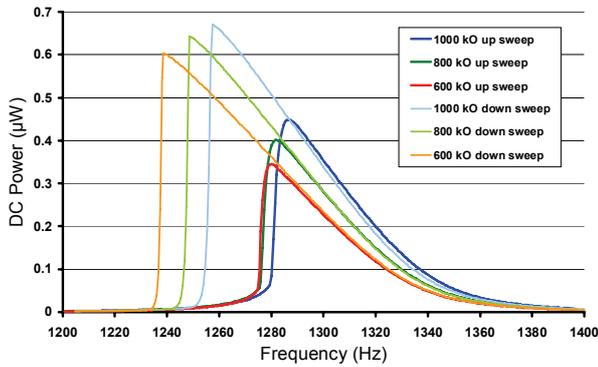
Fig. 9: DC power output for frequency up-sweeps and down-sweeps at different load resistances. Bias voltage: 15 V, Excitation amplitude: 20 m/s<sup>2</sup>
