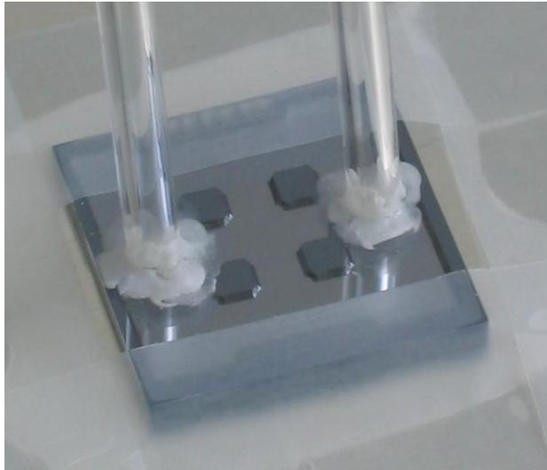
Figure 4. Microfabricated reformer including testing tubes.
