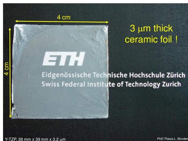
Figure 3. Ultra-thin YSZ ceramic foil prepared by wet ceramic processing.
