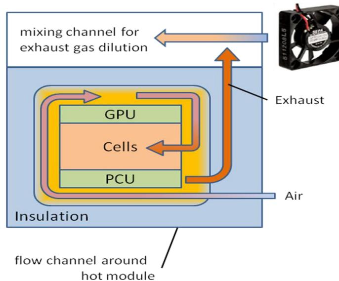
Figure 5. Thermal management concept without exhaust gas heat exchanger.
