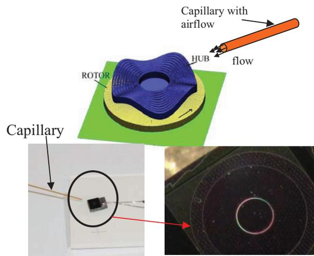
Figure 6. Top: Schematic of Airflow from a pressure vessel being directed to drive a micromotor (not to scale). Bottom right: A micromotor being air driven. Left: An enlarged view of the micro motor with rotor and hub.
