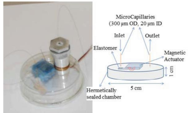
Figure 5: Capillary emerging from the pressure vessel and into the hermetically sealed chamber with magnetic actuator for flow control. Right: Enlarged schematic view of the chamber and magnetic valve.
