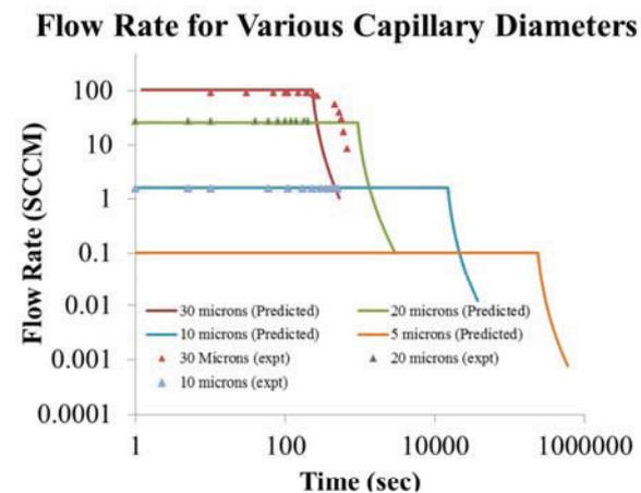
Figure 4. Flow rate as a function of time for 1 gram carbon dioxide in 1-cc vessel for various capillary sizes. Lines represent the predicted flow rate for various diameters. As can be seen flow rate falls rapidly with radius leading to several days of operation for smaller diameter capillaries.
