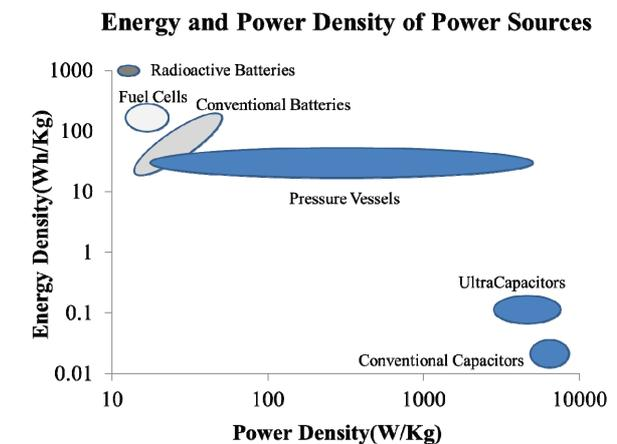
Figure 1. Chart showing the relative merit of various power sources. As can be seen pressure vessels not only having high energy density, but also a wide range of operation for power density due to flexibility in discharge rates.
