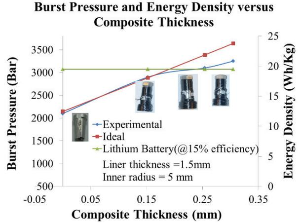
Figure 2. Burst pressures obtained for various composite thicknesses and the energy density of the corresponding vessel. The energy density exceeds lithium batteries at a pressure of 3000 bar
