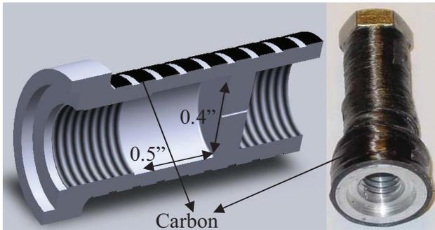
Figure 3. Pressure Vessel Left: A schematic cut section of the pressure vessel showing the chamber and wrapping of Carbon fiber. Right: A wrapped vessel.
