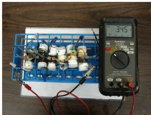
Fig. 2: A string of six cells to generate 3.45 V.
