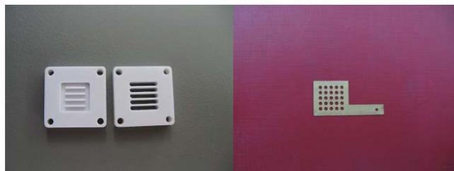
(a) Anode and cathode plate (b) current collector
