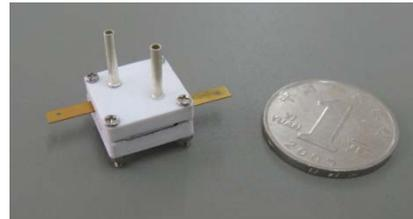
Fig.4: Prototype of  $\mu\text{DMFC}$
