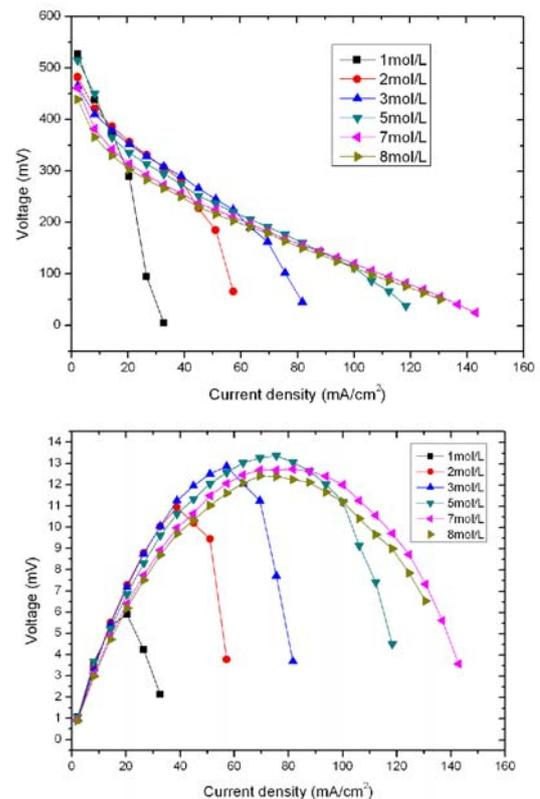
Fig.5: Effect of methanol concentration on the performance of  $\mu\text{DMFC}$
