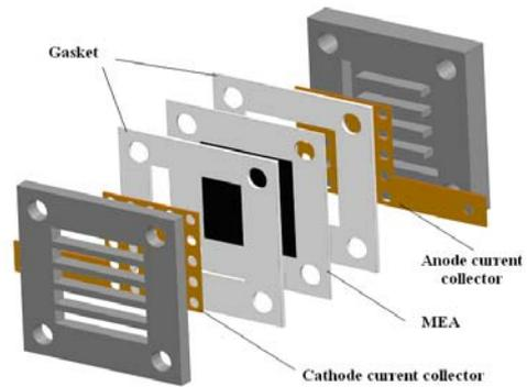
Fig.3: Schematic of  $\mu\text{DMFC}$
