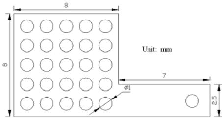
Fig.2: Illustration of current collector
