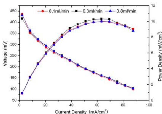
Fig.6: Effect of methanol flow velocities on performance of  $\mu\text{DMFC}$
