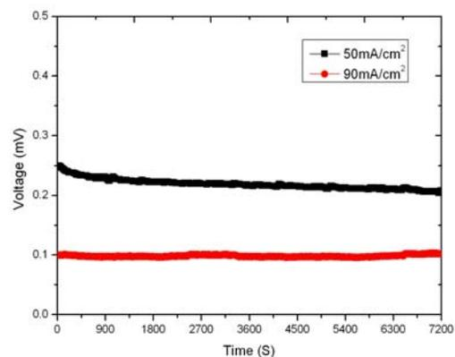
Fig.7: Two-hour performance at  $50\text{mA/cm}^2$  and  $90\text{mA/cm}^2$  using 7mol/L methanol with 0.1ml/min flow velocity
