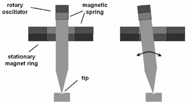
Fig. 4: Illustration of the new design principle of the harvester presented in this paper.
