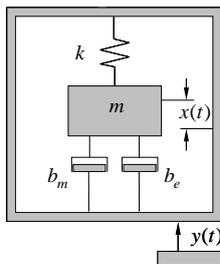
Fig. 1: Schematic sketch of a spring mass system described by equation 1.
