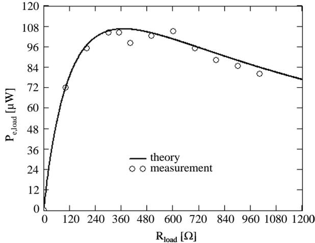
Fig. 6: Electrical output power plotted against the load resistor for the harvester typ1.
