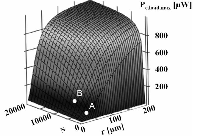
Fig. 3: Calculated maximum electrical output power in dependence on coil turns and coil wire thickness.
