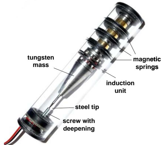
Fig. 5: Photograph of a prototype of the harvester with proposed design. The main features are indicated.
