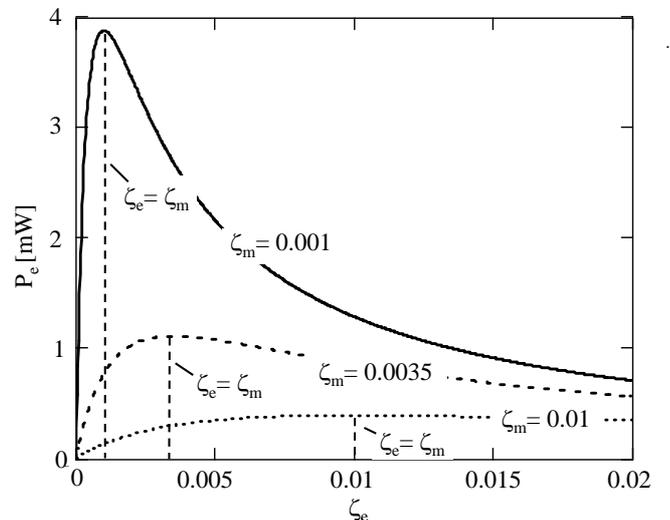
Fig. 2: Electrical output power of a resonantly working energy harvester calculated by equation (2).
