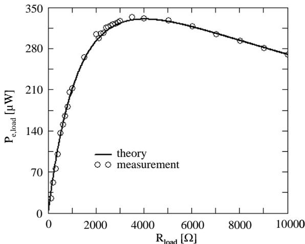
Fig. 8: Electrical output power plotted against the load resistor for the harvester typ2.
