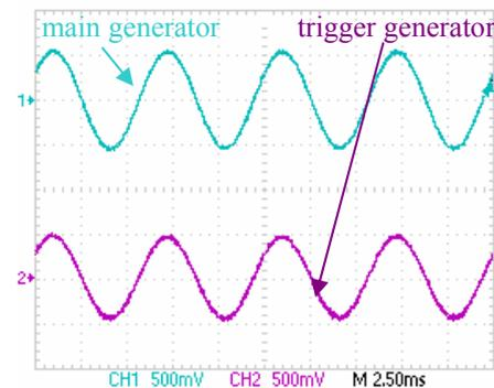
Fig. 10: Voltage output of the trigger and the main generator (mechanical excitation with a vibration amplitude of 0,06g)
