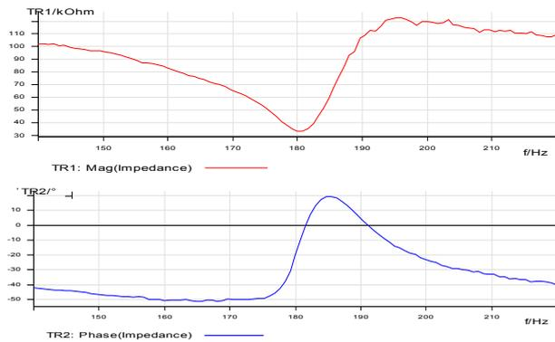
Fig. 8: gain phase measurement of the piezoelectric generator (main electrode)
