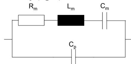
Fig. 7: electrical equivalent circuit of the energy harvester
