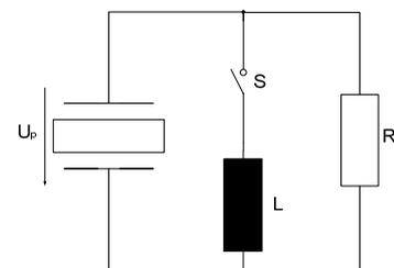
Fig. 2: Simplified model of a SSHI circuit, consisting of piezoelectric harvester, switch, inductor and load resistor
