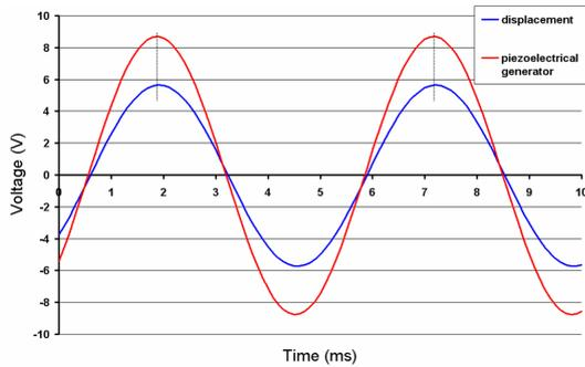
Fig. 3: Measurement of the correlation between output voltage and mechanical displacement of a piezoelectric generator
