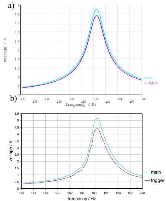
Fig. 6: FEM simulation results (a) and measurement results (b) of the piezoelectric output voltages.
