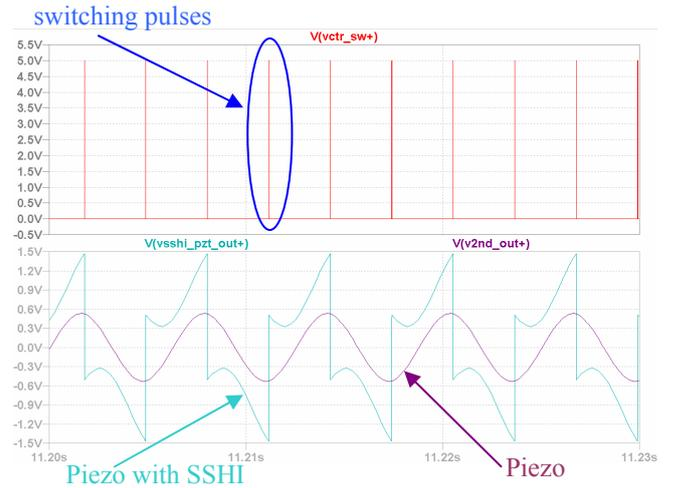
Fig. 9: Simulation results of the output voltages of the piezoelectric energy harvester with and without additional SSHI interface
