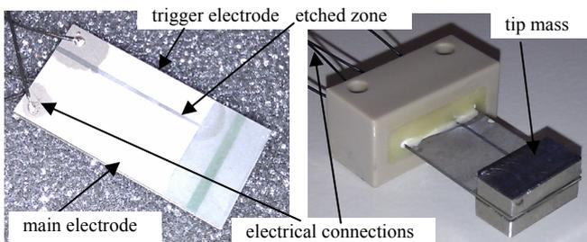
Fig. 4: piezoelectric bimorph with 2 different electrode structures
