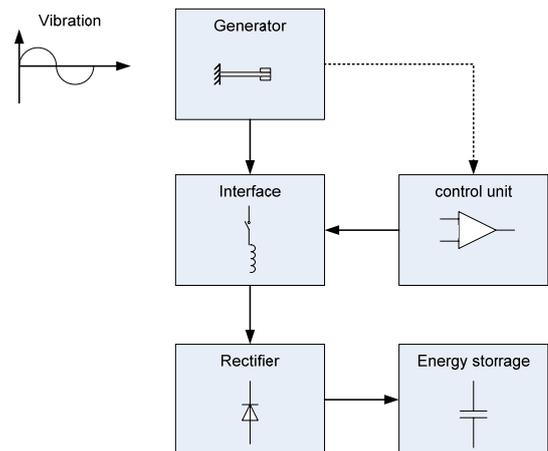
Fig. 1: Energy harvesting device with additional SSHI-Interface and control unit
