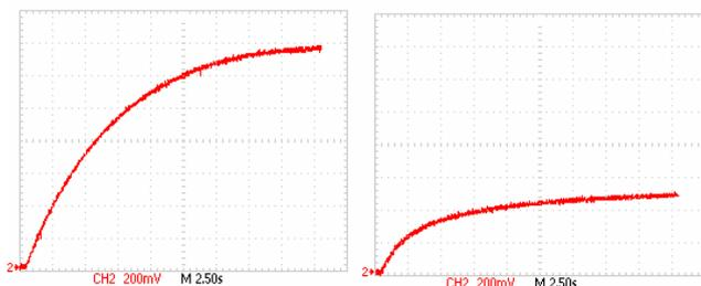
Fig. 13: charging a  $10\mu\text{F}$  capacitor with (a) the piezoelectric generator with SSHI circuitry (b) the piezoelectric generator without SSHI circuitry
