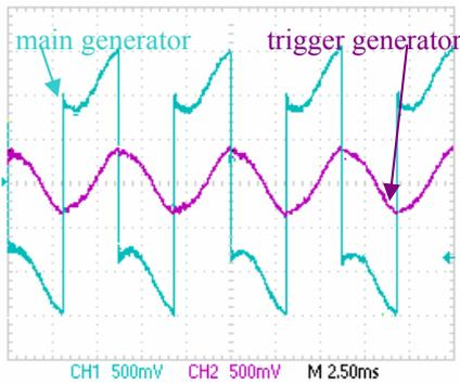
Fig. 11: Voltage output of the trigger and the main generator with additional SSHI interface. (mechanical excitation with a vibration amplitude of 0,06g)
