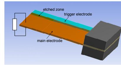
Fig. 5: FEM-Model of the piezoelectric generator
