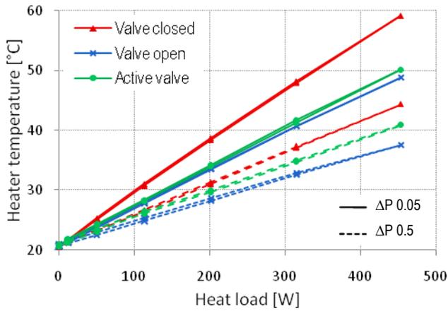
Figure 9: Heater temperature versus heat load.
