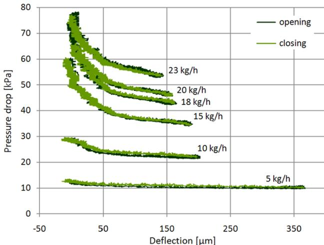
Figure 11: Pressure drop versus deflection.
