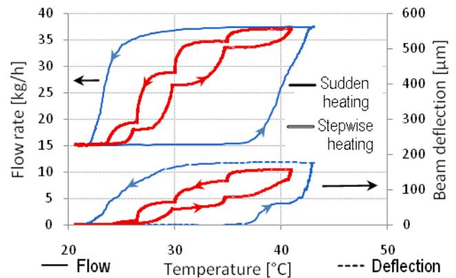
Figure 7: Flow rate and beam deflection vs. temperature at a  $\Delta P$  of 0.5 bar.
