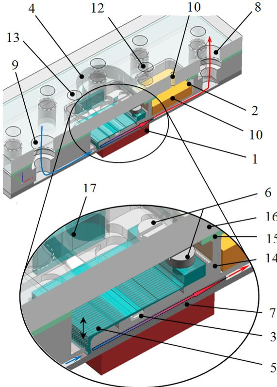
Figure 3: Section view of the thermopneumatic valve.
