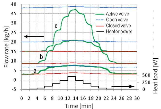
Figure 8: Flow rate in function of time for a stepped heat input at  $\Delta P$  0.05 (a), 0.2 (b) and 0.5 bar (c).
