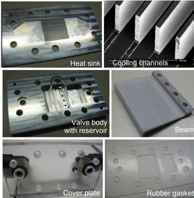
Figure 5: Thermopneumatic valve components.
