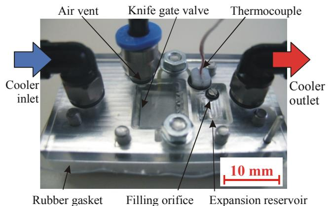
Figure 1: Assembled thermopneumatic valve.
