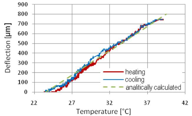
Figure 6: Beam deflection versus temperature at atmospheric pressure.
