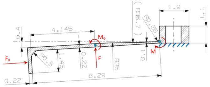
Figure 4: Cross-section of the designed beam.
