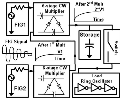
Figure 8. A preliminary power management system is assembled on a breadboard. Each FIG is connected to a 6-stage Cockroft-Walton multiplier. The output of these multipliers is cascaded and stored on a capacitor. The charged capacitor can be used to power a ring oscillator.
