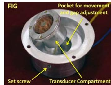
Figure 4. Photograph showing a close-up of the fabricated FIG and movable transducer.
