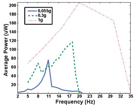
Figure 7. Frequency response of the PFIG generator at different vibration amplitudes. The PFIG generator is able to operate over an unprecedented acceleration range of nearly 2 orders of magnitude.
