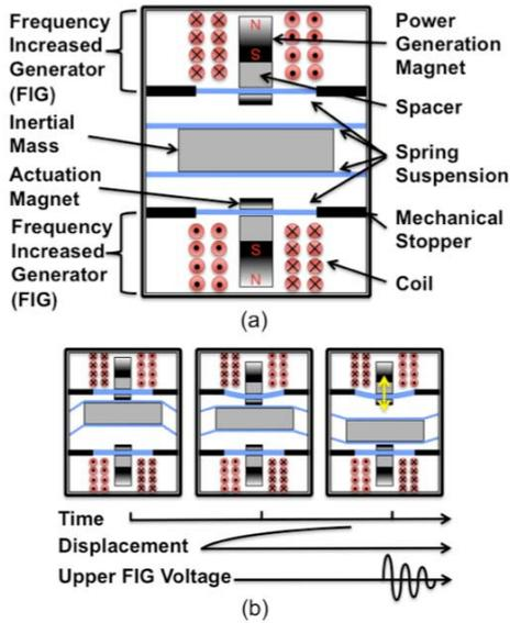
Figure 2. a) Parametric Frequency Increased Generator (PFIG) architecture b) Illustration of the method of operation.
