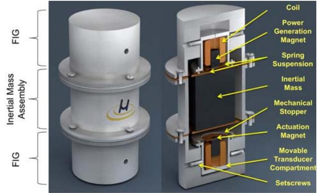
Figure 3. Conceptual diagram of the bridge harvester implementation. The WC inertial mass is suspended on two copper springs in the middle. The FIGs are shown on top and bottom, clamped using setscrews inside a holding fixture.
