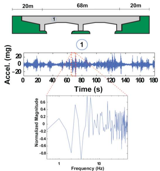
Figure 1. Vibration data from a typical bridge showing the amplitude of the acceleration as well as the frequency response of the waveform. The traffic-induced vibrations are very small in amplitude and low in frequency.
