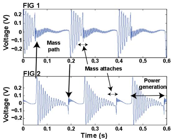
Figure 6. Oscilloscope recording showing the parametric generator operation from 55mg at 5 Hz. The top and bottom voltage waveforms correspond to the top and bottom FIG devices as the inertial mass snaps back and forth between them.
