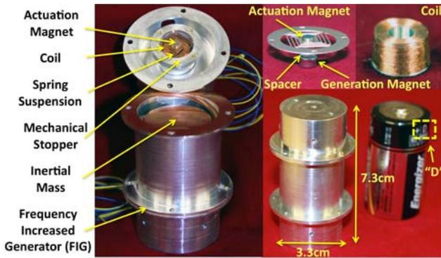
Figure 5. Photographs showing the completed PFIG. On the left, the device is opened exposing the internal components. The electromagnetic transducer components are shown on the top right. The completed PFIG is shown alongside a standard “D” size battery on the bottom right.
