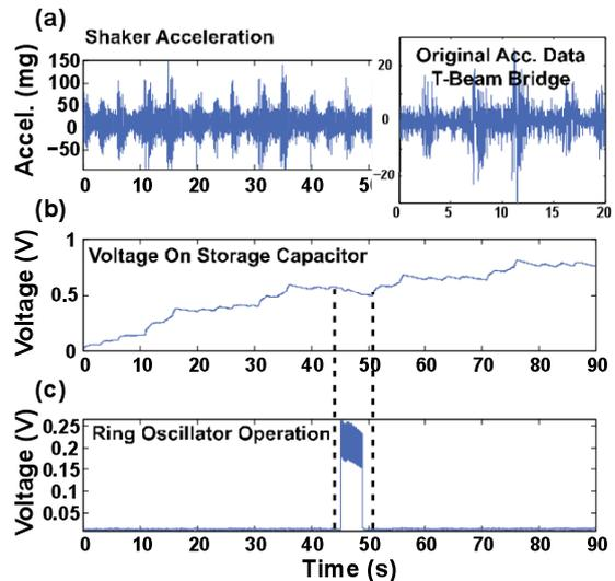
Figure 9. The PFIG can scavenge non-periodic wide-band vibrations. a) A recording of the acceleration used to drive the PFIG (this is an amplified signal measured on a highway flyover bridge). b) Voltage of the storage capacitor rising over time. c) Unregulated power is used to drive the ring oscillator.
