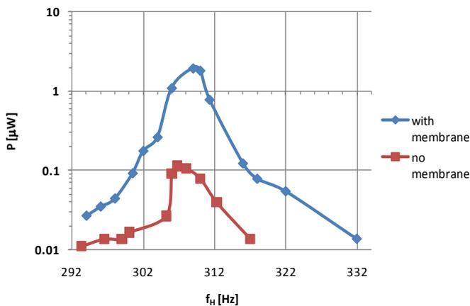
Fig. 5: Power generated by the piezoelectric harvester at  $R_0 = 3.3 \text{ M}\Omega$ , constant airflow velocity of 13 m/s and changing volume of the cavity of the Helmholtz resonator.
