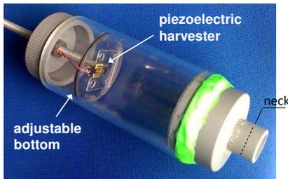
Fig. 2: Photograph of the Helmholtz resonator with the piezoelectric cantilever harvester in it.
