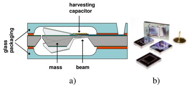
Fig. 4: a) Vibration energy harvester packaged in between glass substrates. The mass can move up- and downwards; b) Photograph of various piezoelectric energy harvesters.
