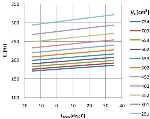
Fig. 9: Dependence of the frequency of the Helmholtz resonator on the temperature of the air at fixed volume of the cavity. Calculated using eqn. (1).
