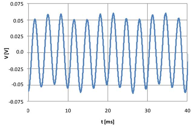
Fig. 7: Output voltage in time of the piezoelectric harvester mounted in the Helmholtz resonator with membrane, at  $R_0 = 3.3 \text{ M}\Omega$ ,  $f_p = 309 \text{ Hz}$ , airflow velocity of 13 m/s.
