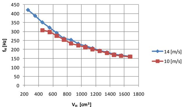
Fig. 3: Dependence of the frequency of the custom Helmholtz resonator on the volume of the cavity at constant airflow velocity. Measured with Helmholtz resonator presented in Fig 2.
