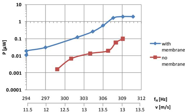
Fig. 6: Power generated by the piezoelectric harvester at  $R_0 = 3.3 \text{ M}\Omega$ , constant volume of the cavity of the Helmholtz resonator and different airflow velocities.
