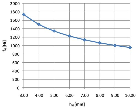
Fig. 8: Dependence of the frequency of the Helmholtz resonator on the height of the cavity  $h_H$  at fixed temperature 25°C. The neck has dimensions 5 mm x  $\varnothing$  3mm. The cavity has diameter  $\varnothing$  2cm.
