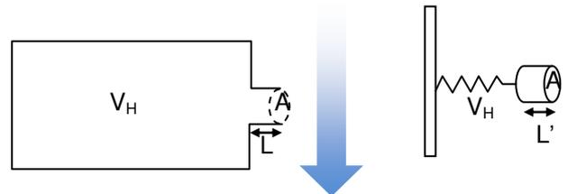
Fig. 1: Helmholtz resonance cavity and a mass-spring representation.
