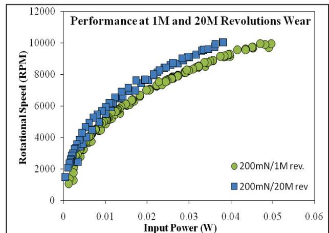
Figure 2 Performance comparison for a MTD tested under 200mN normal loads at 1Mrev. and 20Mrev. running time .
