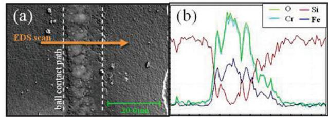
Figure 4 (a) Scanning Electron Microscope images of characteristic wear for silicon, raceways. EDS line scans taken perpendicular to the wear track presented in (b), correlating with the adjacent SEM image.
