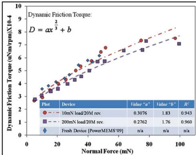
**Figure 5** The results of spin-down friction testing of devices after 20Mrev. wear compared with a previously reported silicon turbine[11].
