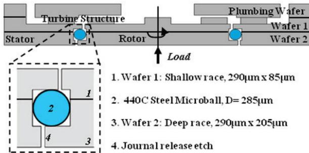
Figure 1 Cross section schematic of the microturbine tribology test device with a close-up of the raceway.
