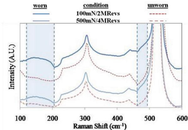
Figure 3 Raman Spectra from two silicon raceways with different contact pressures and lifetimes.
