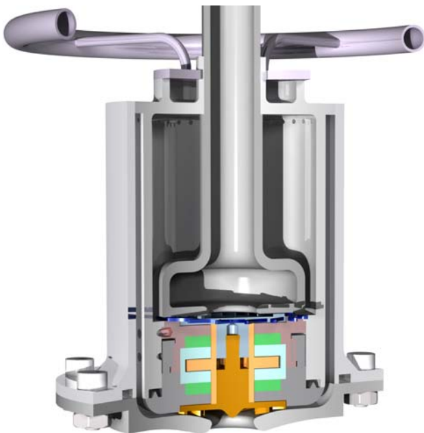
Figure 1 - Ultra micro gas turbine concept.
