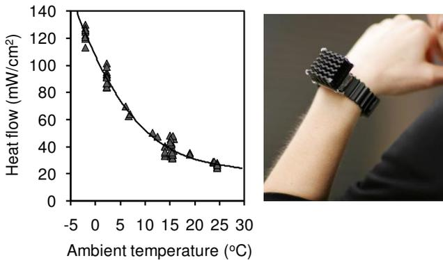
Fig. 2: Dependence of the heat flow in the wrist on ambient temperature measured on a standing or sitting person by using a TEG with a radiator, and its photo.
