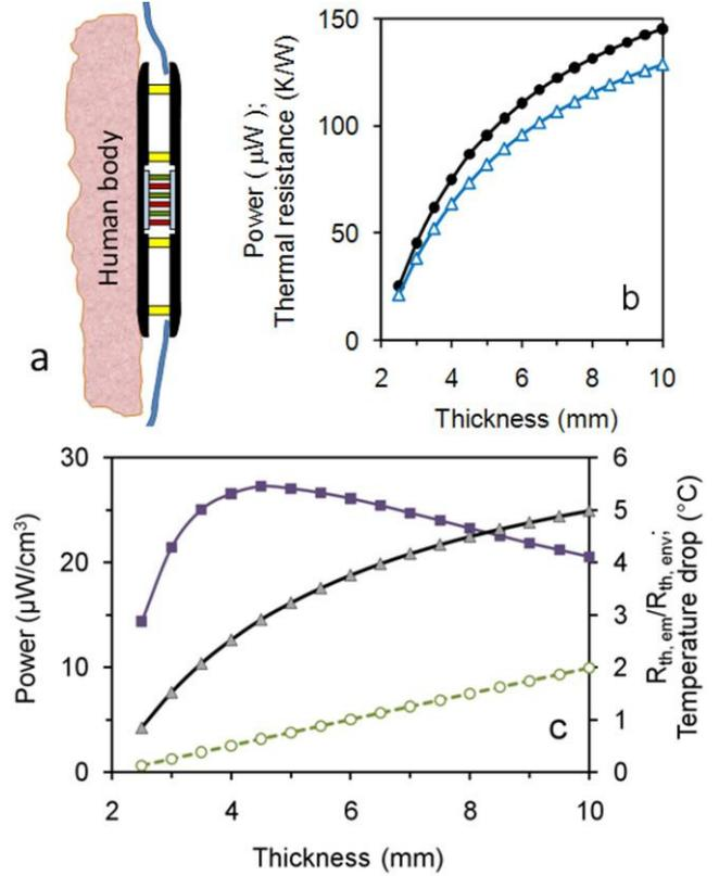
Fig. 5: (a) Design of the simulated TEG on the body, (b) Simulated dependence of the maximum power (circles) and optimal thermal resistance of the thermopile (triangles), and (c) Simulated dependence of the optimal temperature drop on the thermopile (triangles), the ratio of thermal resistances of "empty" TEG to the environment (circles), and the power per unit volume (squares) on thickness of the TEG.
