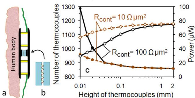
Fig. 7: Simulated (a) TEG with (b) a thermopile, and (c) The dependence of number of thermocouples (circles) needed to reach 0.5 V on the matched load and maximum power at different contact resistance.
