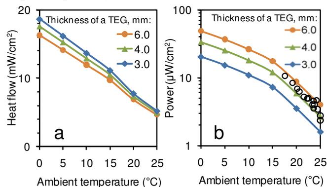
Fig. 6: Simulated dependence of (a) heat flow in the TEG of different thickness, and (b) power on temperature. Open circles show the average power measured in the 6.5 mm-thick TEG of an ECG shirt [3].
