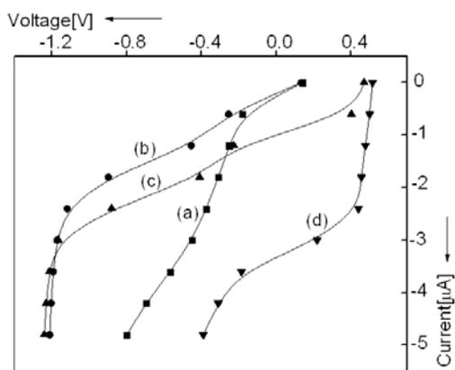
Fig.5. Polarization curve of ABTS as mediator in electrolyte (PBS pH 7.2) (a) 1 mM ABTS+air (b) 1 mM
