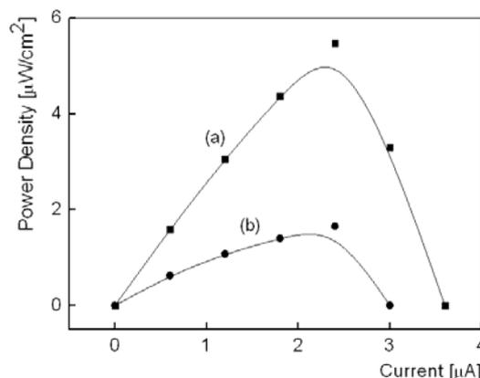
Fig.7. Comparative performance of cells with different mediators(a) Anode:1mM Phenazine as mediator and 10mM Glucose; Cathode:1mM ABTS (b) Anode:1mM Ferrocene as mediator and 10mM Glucose; Cathode:1mM ABTS.
