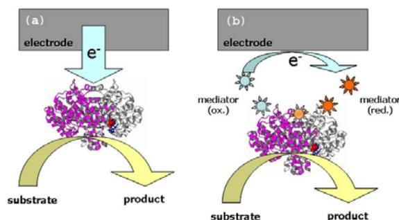
Fig.1. Types of electron transfer pathway. (a) Direct electron transfer (DET). (b) Mediated electron transfer (MET).
