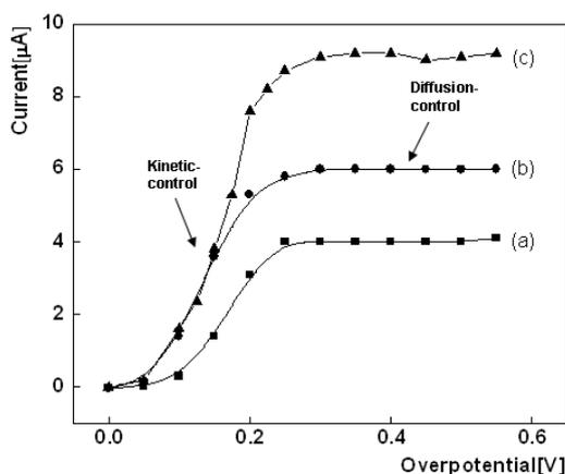
Fig. 4. Potential-step curves at a glassy carbon electrode in a buffered electrolyte (PBS pH 7.2) containing 1 mM Ferrocene as mediator. (a) Ferrocene+Gox; (b) Ferrocene+Gox +10 mM Glucose; (c) Ferrocene+Gox+20 mM Glucose.
