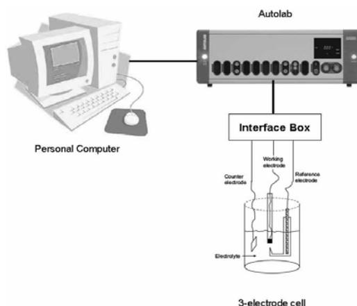
Fig. 2. Schematic representation of the bio-fuel cell testing system.
