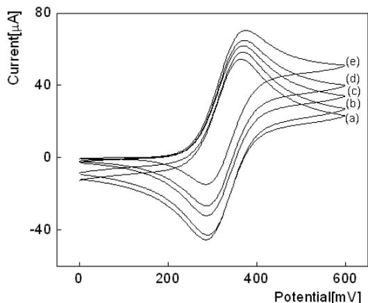
Fig. 3. Cycl.voltammograms at a glassy carbon electrode in a buffered electrolyte (PBS pH 7.2) containing 1 mM Ferrocene as mediator; (a) Ferrocene+Gox; (b) Ferrocene+Gox +10 mM Glucose; (c) Ferrocene+Gox +20 mM Glucose; (d) Ferrocene+Gox +30 mM Glucose; (e) Ferrocene+Gox +40 mM Glucose.
