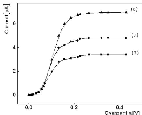
Fig.9. Simulation of current-voltage curves of a BFC system in a buffered electrolyte (PBS pH 7.2) containing 1 mM Ferrocene as mediator. (a) Ferrocene+Gox +1 mM Glucose; (b) Ferrocene+Gox +10 mM Glucose; (c) Ferrocene+Gox +20 mM Glucose.
