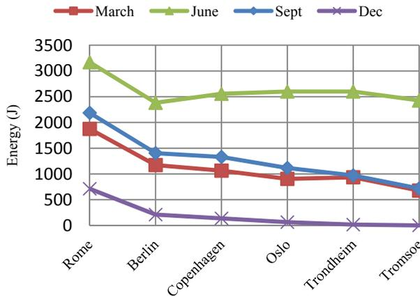
Fig. 4: Daily usable energy produced by a credit card sized silicon solar panel as function of locations and season.
