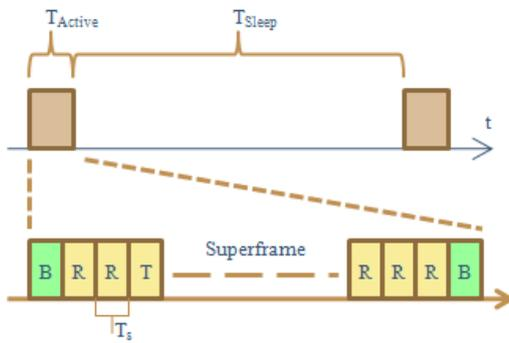
Fig. 2: Active sleep period with a superframe containing beacons (B), receive periods (R) and one transmit period (T).
