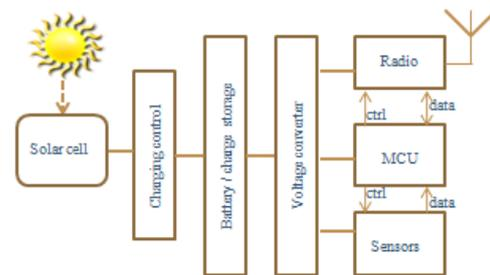
Fig. 1: Block diagram of a typical WSN node.
