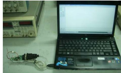
Fig. 4: The photo of the wireless sensor receiving node and interface window.
