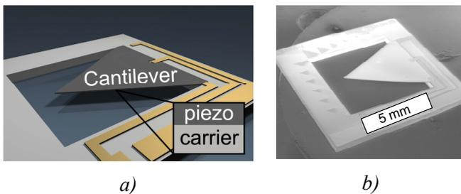
Fig. 3: MEMS piezo cantilever generator: a) device schematic showing the triangular cantilever consisting of the piezoelectric and carrier layer, b) SEM photograph of a realized test structure.
