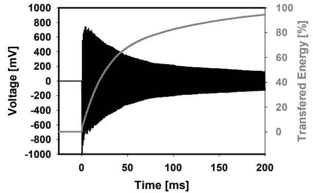
Fig. 4: Pulsed excitation of MEMS generator structure according to Fig. 3. At  $t = 0$  the cantilever is loaded with external mechanical energy. The black line shows the measured transient behavior of the generated voltage and the gray line indicates the amount of transferred energy over time.
