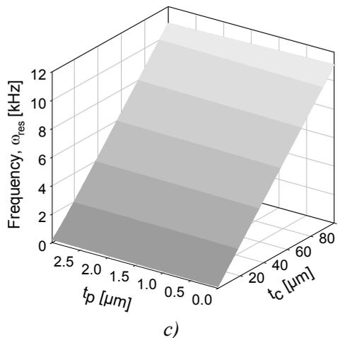
Fig. 6: Examples for calculated system parameters: power, voltage and natural frequency, displayed over the geometry design space (area is fixed to 25 mm<sup>2</sup>).
