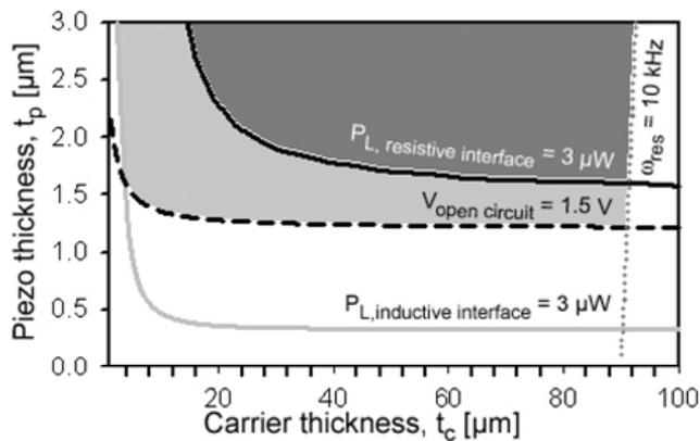
Fig. 7: System parameter contour lines on generator design space. Resistive interface schemes require geometries in dark grey area. Requiring a minimum open circuit voltage of  $1.5 V$  the inductive interface schemes allow for additional design space in the light grey region.
