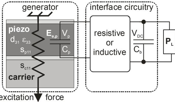
Fig. 2: System components of the piezoelectric energy harvesting module. The generated electrical energy  $E_{e,p}$  is provided through the interface circuit as load power  $P_L$ .
