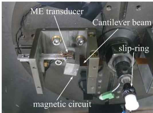
Fig. 5: Photograph of the proposed energy harvester.
