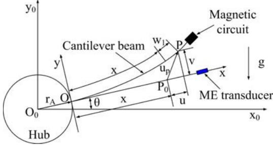
Fig.2: Structural model of the hub-beam system
