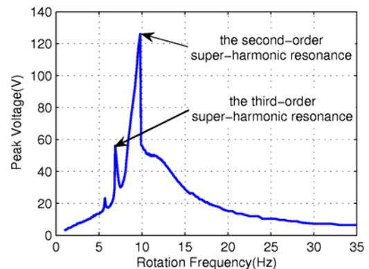
Fig.7: Measured peak voltage free of load versus rotation frequency
