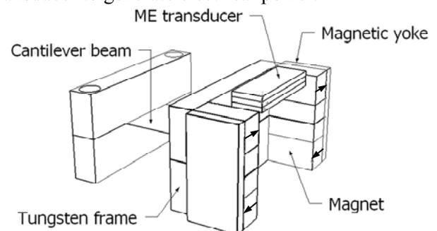
Fig.1: Schematic diagram of the proposed harvester.
