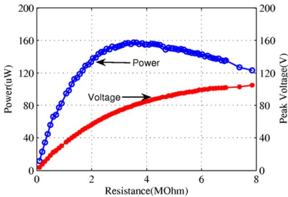
Fig.9: Experimental power and voltage versus load resistance.
