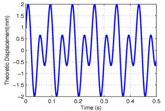
Fig.3: Prediction of the transverse displacement of the magnetic circuit versus time at the second-order super-harmonic resonance
