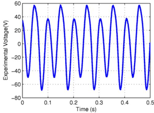
Fig.8: Measured peak voltage free of load
