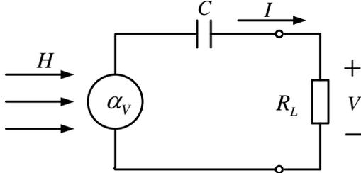
Fig.4: ME transducer equivalent circuit
