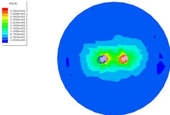
Fig. 3: The magnetic field distribution surrounding a cord consisting of two wires carrying identical currents in opposite direction
