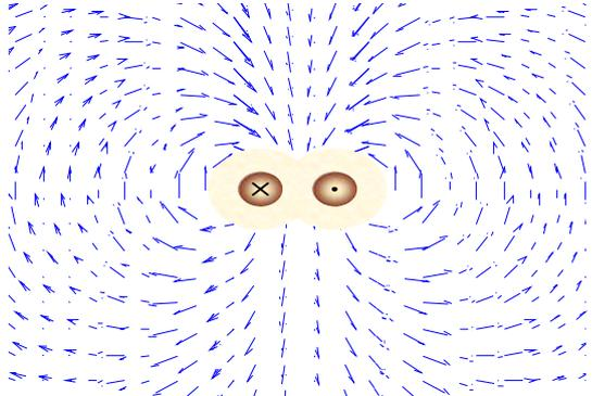
Fig. 2: The magnetic field in a plane perpendicular to a cord consisting of two wires carrying identical currents in opposite direction
