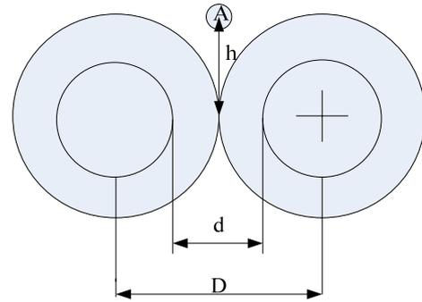
Fig. 4: Measurement of magnetic field from a cord consisting of two wires carrying identical currents in opposite directions
