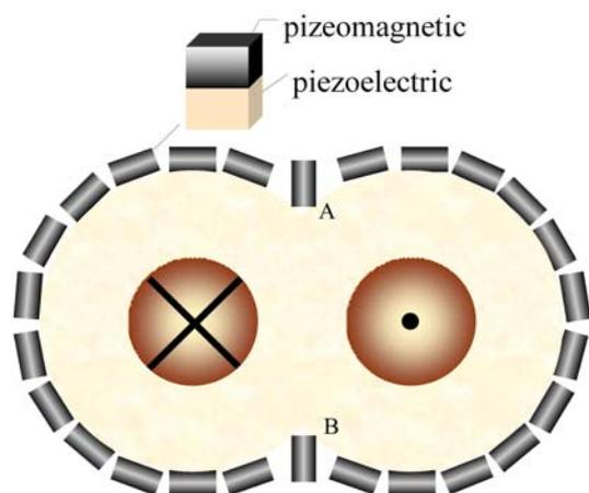
Fig. 5: The schematic configuration of composite ME transducers for scavenging the ac magnetic field surrounding an appliance cord
