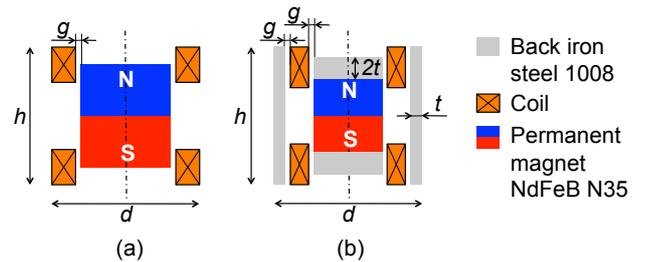
Figure 2. Analyzed cylindrical setups with (a) and without (b) back iron
