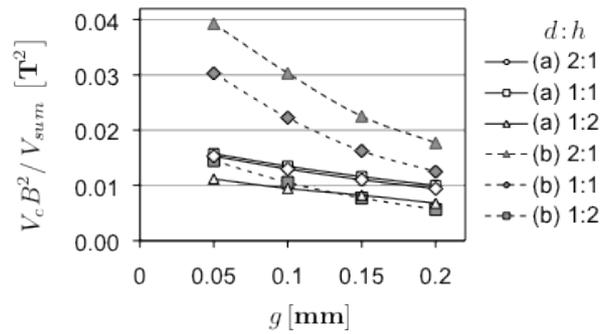
Figure 3.  $V_c B^2 / V_{sum}$  with respect to the airgap  $g$  and the aspect ratio  $d:h$  for setup (a) and (b).
