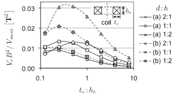
Figure 6.  $V_c B^2 / V_{sum}$  with respect to the ratio of the coil thickness  $t_c$  to height  $h_c$  and the aspect ratio  $d:h$  for setup (a) and (b) at an airgap  $g = 0.1$  mm.
