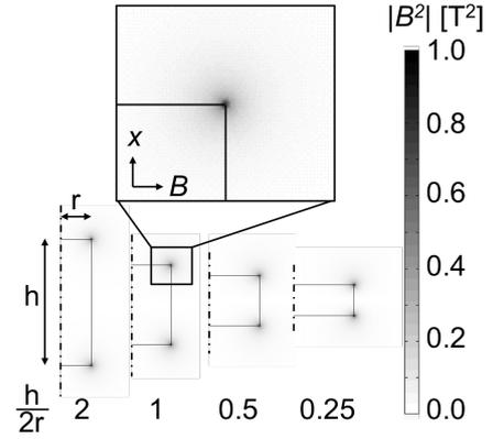
Figure 5. Distribution of  $B^2$  of cylindric magnets with different aspect ratio.
