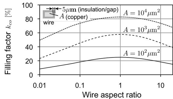
Figure 4. Filling factor with respect to the coil aspect ratio and the wire cross section  $A$  for an insulation thickness or half gap width of 5  $\mu\text{m}$ .
