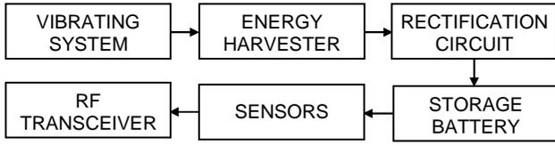
Fig. 1: Schematic of the self-powered network node for applications in rail vehicles.
