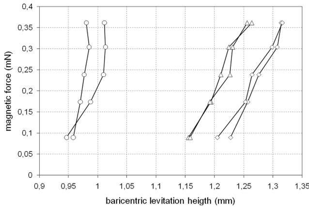
Fig. 6: Magnetic force calculated from the static equilibrium of proof masses with different thicknesses and one ( $\circ$ ), two ( $\triangle$ ) or three ( $\diamond$ ) layers of NdFeB permanent magnets.
