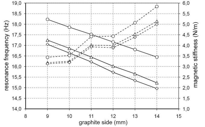
Fig. 7: Resonance frequency (continuous) and dynamic magnetic stiffness (dashed) of the suspension with one ( $\circ$ ), two ( $\triangle$ ) or three ( $\diamond$ ) layers of NdFeB permanent magnets.
