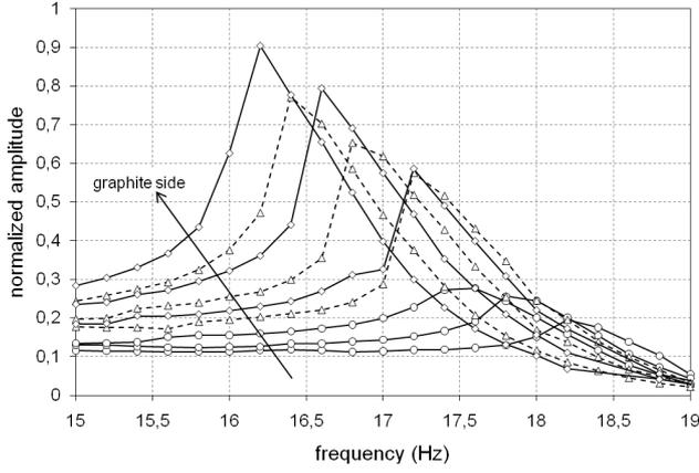
Fig. 5: Dynamic response of the suspension for 9, 10 and 11mm graphite side with one ( $\circ$ ), two ( $\triangle$ ) or three ( $\diamond$ ) layers of NdFeB permanent magnets.
