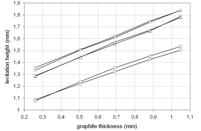
Fig. 3: Levitation height of graphite with variable thicknesses with one (○), two (△) or three (◇) layers of NdFeB permanent magnets.
