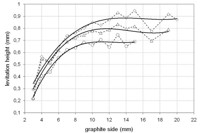
Fig. 4: Levitation height of graphite with variable side lengths with one (○), two (△) or three (◇) layers of NdFeB permanent magnets.
