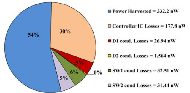
Fig. 7: Power budget for synchronous electrostatic energy harvesting IC
