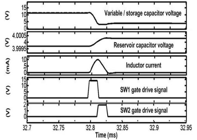
Fig. 6: Voltage and current waveforms for proposed structure during flyback of energy.
