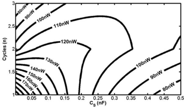
Fig. 2: Power harvested as function of cycle and storage capacitor value for traditional asynchronous architectures.
