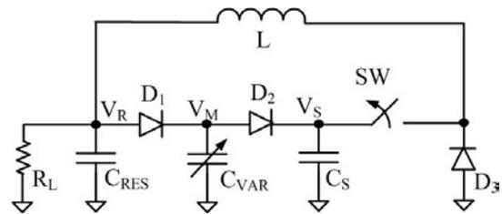
Fig. 1: Asynchronous energy harvesting circuit.
