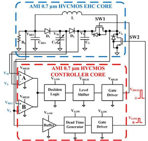
Fig. 3: AMI 0.7 $\mu$ m EHC Core (blue) and Controller IC Core (red).
