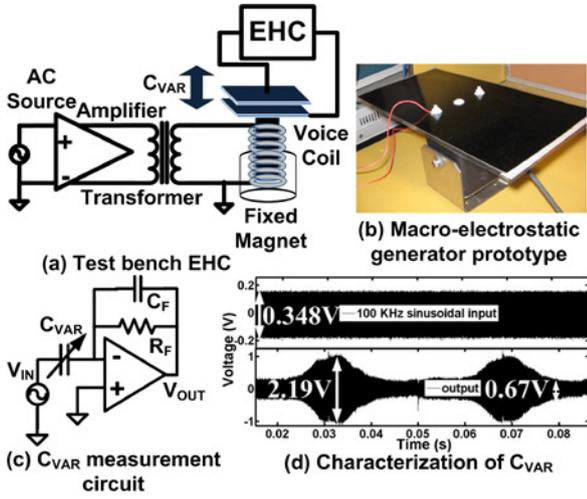
Fig. 4: (a) Experimental setup for testing the energy harvesting circuit with macro variable capacitor prototype, (b) Macro generator prototype (c) Circuit for direct measurement of variable capacitance, (d) Measured capacitance variation of electrostatic generator.
