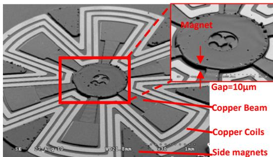
Fig 6 : SEM photo of the harvester
