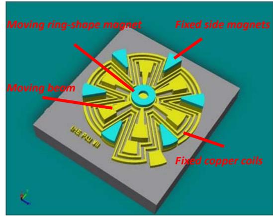
Fig 2 : Micro electromagnetic energy harvester
