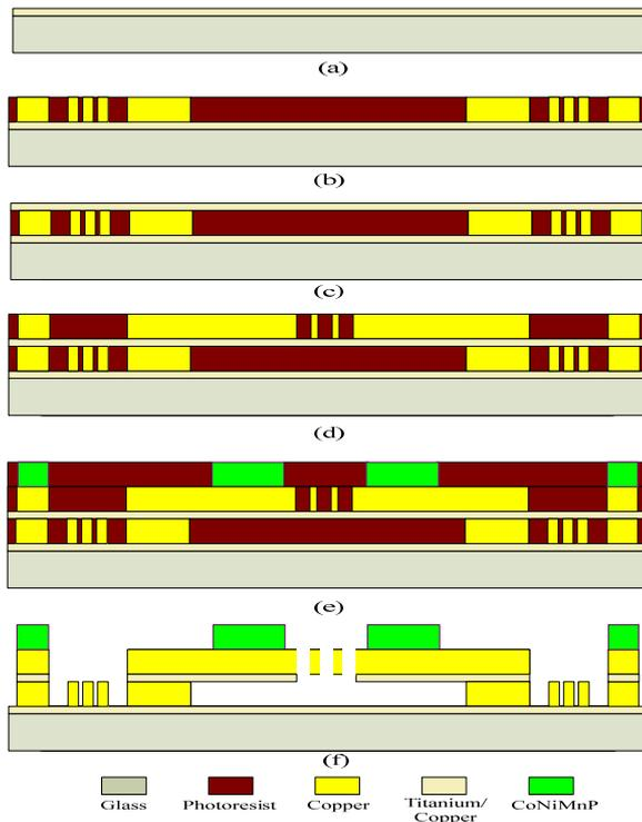
Fig 5 : Illustration of Fabrication process
