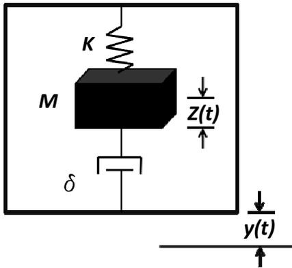
Fig 1 : Model of a spring-mass energy harvester
