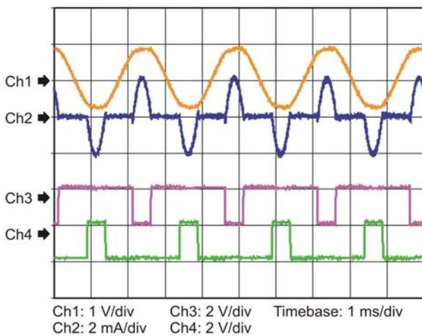
Fig. 6: Scope traces showing power conditioner input voltage (Ch1) and current (Ch 2), and gate drive signals applied to M2/M3 (Ch3) and M1/M4 (Ch4).
