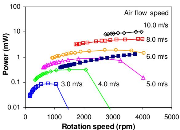
Fig. 9: Variation with rotation speed of (a) measured turbine output power at different air flow speeds (open symbols), and (b) input power requirement of power conditioner (filled symbols).
