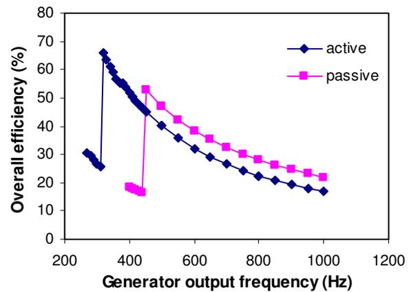
Fig. 5: Conversion efficiencies of conditioner in passive and active modes as a function of generator output frequency.
