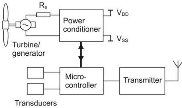
Fig. 3: Block diagram of complete wireless sensor.
