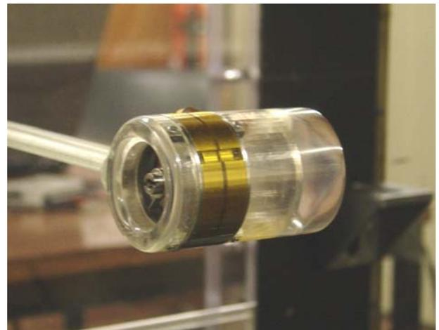
Fig. 2: Prototype turbine installed in the experimental section of an 18'' x 18'' wind tunnel.
