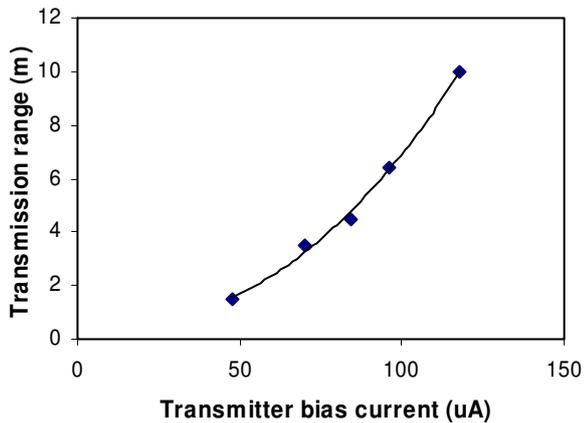
Fig. 8: Measured variation of transmission range with bias current for Colpitts oscillator transmitter.
