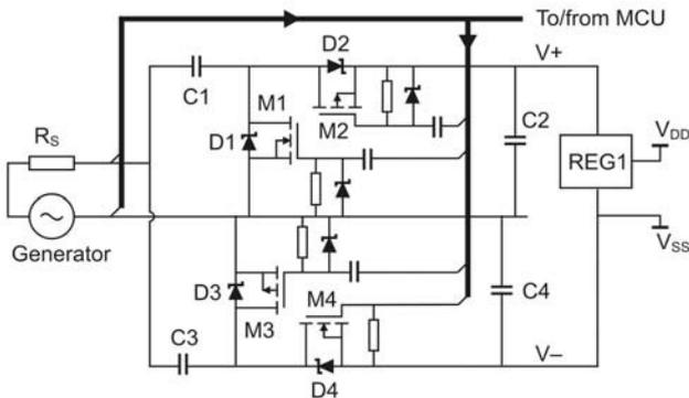
Fig. 4: Power conditioning block based on 2-sided, synchronous voltage doubler.
