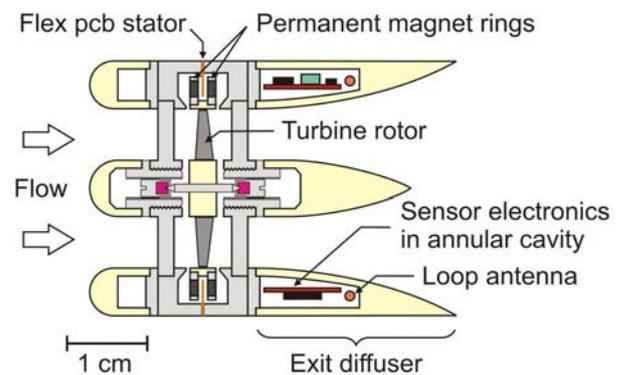
Fig. 1: Schematic cross-section of sensor showing turbine/generator geometry and cavity for electronics.
