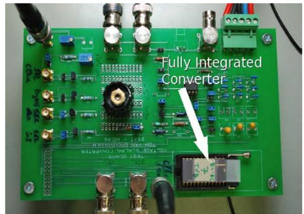
Fig. 10: PCB realization of the Test Bench
