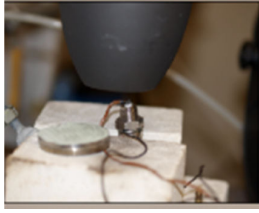
Figure 8 - IR lamp test setup. The modified sparkplug with a surface mounted thermoresistor.
