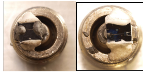
Figure 5 – Image of Pt thermoresistor mounted to a sparkplug with Ni resbond used as electrical contact (left) and Al wirebonds connect the sensor (right).
