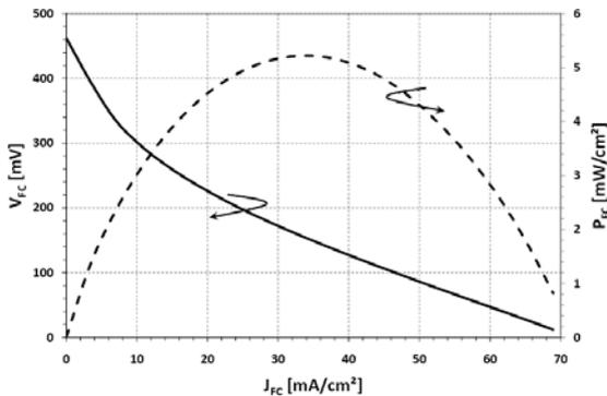
Fig. 3: Voltage vs. current density ( $V_{FC}$ - $J_{FC}$ ) and power density vs. current density ( $P_{FC}$ - $J_{FC}$ ) characteristics measured on the  $\mu DMFC$  micro fuel cell operated with 2M-methanol.
