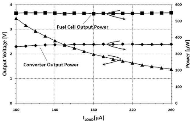
Fig. 8: Power supplied by both the micro fuel cell and the whole power supply module are plotted versus the load current  $I_{LOAD}$  along with the converter output voltage when  $V_{FC}=300mV$ .
