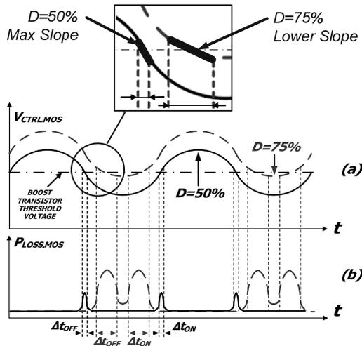
Fig. 5: Switching power losses on MOSFET driven by sinusoidal signal with duty cycle  $D=50\%$  and  $D=75\%$
