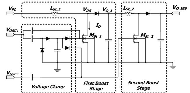
Fig. 4: Schematic of the Intermediate DC-DC boost converter- IBS.
