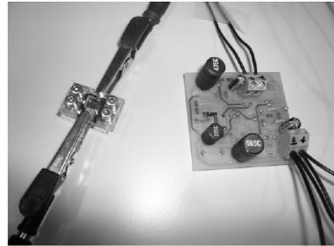
Fig. 6: Picture of the complete power supply module comprised of micro fuel cell and boost converter
