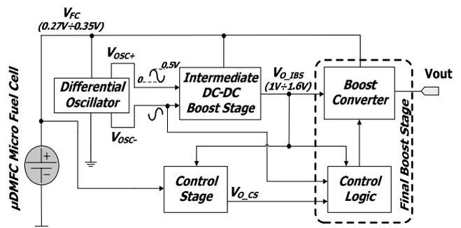
Fig. 1: Block Diagram of the proposed Micro Power Supply Module
