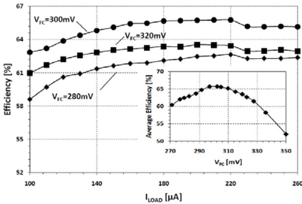
Fig. 7: Boost converter efficiency plotted versus the load current  $I_{LOAD}$ . The inset shows the average efficiency of the boost converter plotted versus the micro fuel cell operating point.
