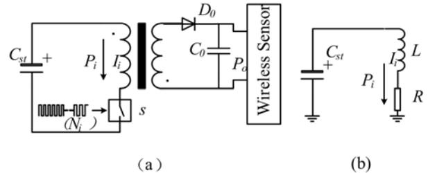
Fig. 7: Fly-back power instantaneous discharged circuit.
