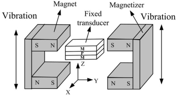
Fig. 1: Vibrating transducer structure.
