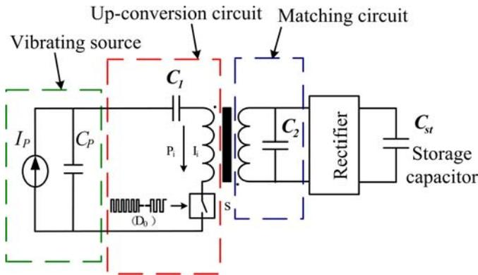
Fig. 5: Frequency-changeable matching circuit.
