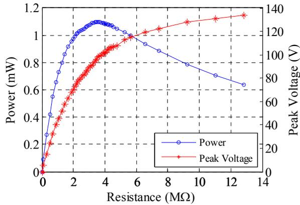
Fig. 2: Output power and voltage as a function of load resistance.
