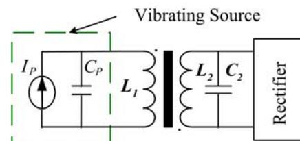
Fig. 4: Traditional transformer matching circuit.
