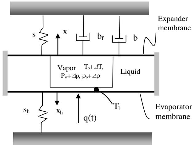
Fig. 2: Model schematic of the micro heat engine.
