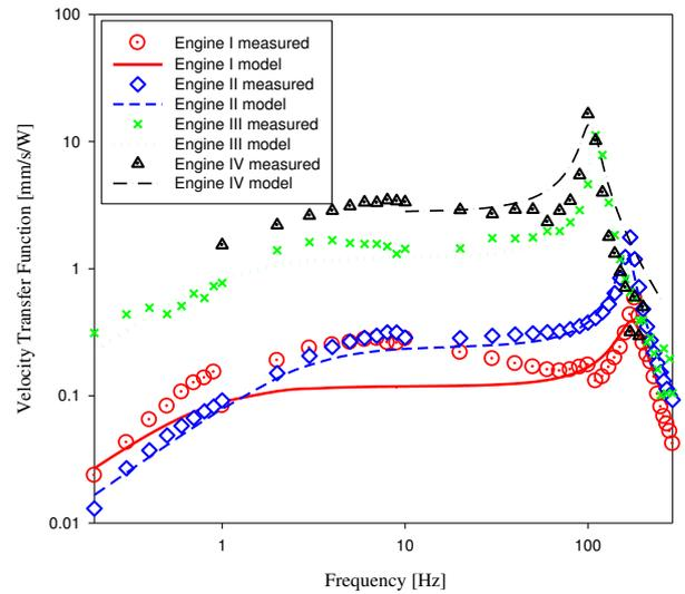
Fig.3: Velocity transfer functions of the tested engines.
