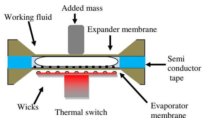
Fig. 1: Schematic of the micro heat engine.
