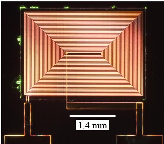
Fig. 5: A completed planar spiral micro-coil to be employed as a passive part of the electromagnetic transducer for vibration energy harvesting.
