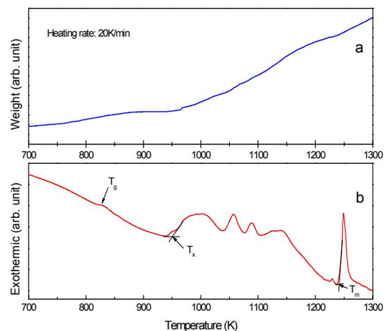
Fig. 2: TGA (a) curve and DSC (b) curve of the 4.5  $\mu\text{m}$  thick FeBNbNd magnetic metallic glass film.
