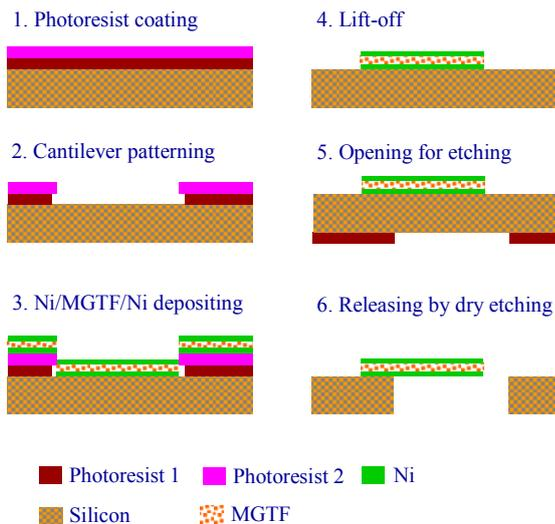
Fig. 1: A fabrication process diagram of a micro-cantilever made of the FeBNbNd metallic glass film with nickel protective layers.
