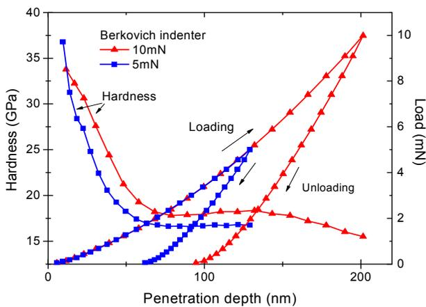
Fig. 3: Loading – unloading curves and respective hardness values as a function of penetration depth of the FeBNbNd metallic glass film were obtained by performing nanoindentation testing using the Berkovich indenter applied maximum loads of 5 mN and 10 mN.
