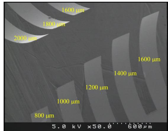
Fig. 4. An SEM image of the magnetic freestanding micro-cantilevers with different lengths (designated in the image for each micro-cantilever).
