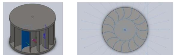
Fig. 1 Rotor isometric and top view
