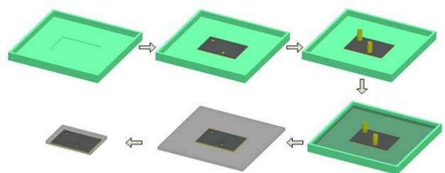
Fig. 2 Schematic of the Encapsulation process using PDMS
