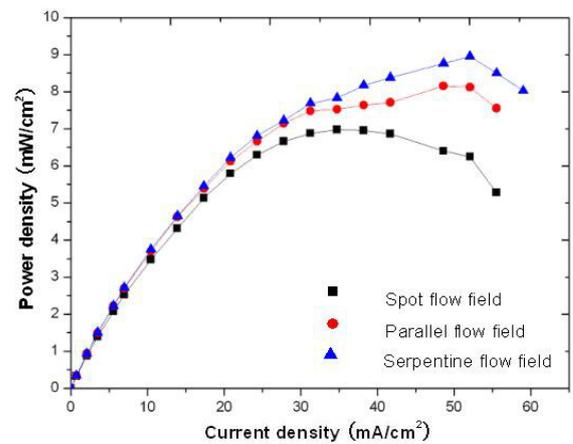
Fig.6 Performance curve of micro DMFCs with different anode flow fields
