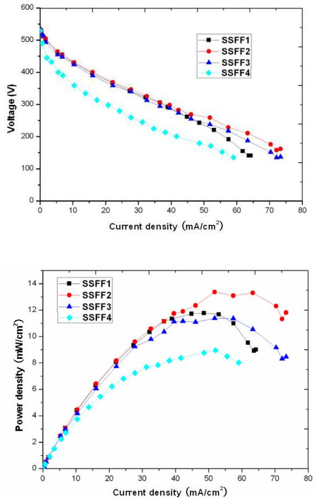
Fig.7 Performance curve of micro DMFCs with different duty cycle
