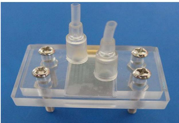
Fig.4 Silicon-based DMFC
