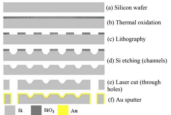
Fig. 1 Schematic of the fabrication process of the silicon-based current collector
