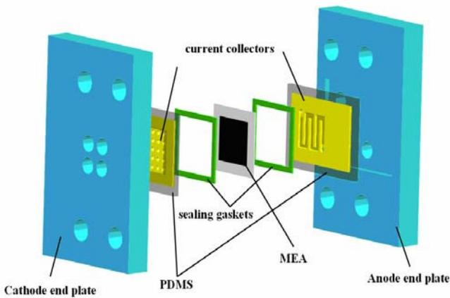
Fig. 3 Schematic of the  $\mu$ DMFC structure
