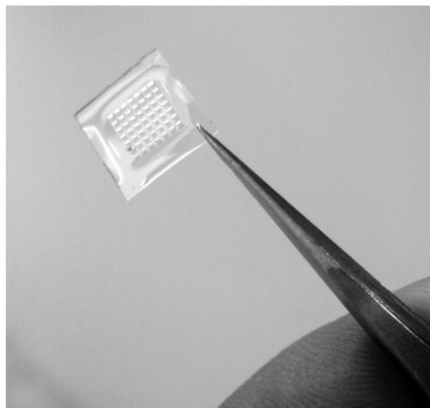
Fig. 4: Picture of one of the microfabricated PDMS membranes.
