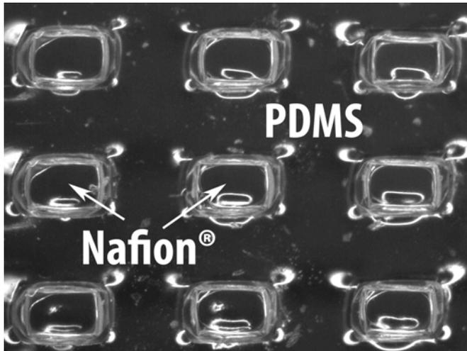
Fig. 5: Detail of the hybrid PDMS-Nafion<sup>®</sup> membrane.
