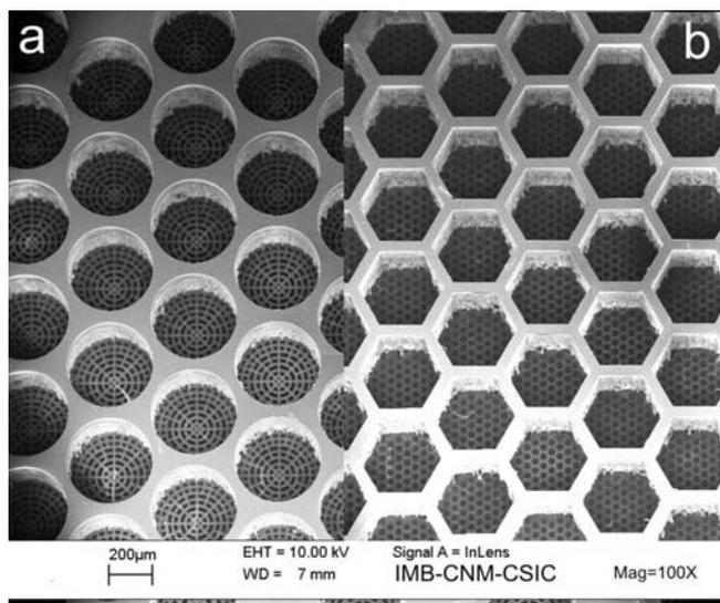
Fig. 3: SEM image of two designs (a-circular and b-hexagonal) of the microfabricated current collectors. Image has been taken from the back side of the silicon chips.
