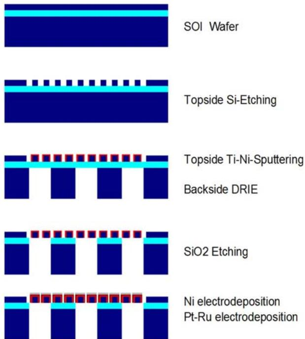
Fig. 2: Main steps of the fabrication process of electrode-current collector structure.
