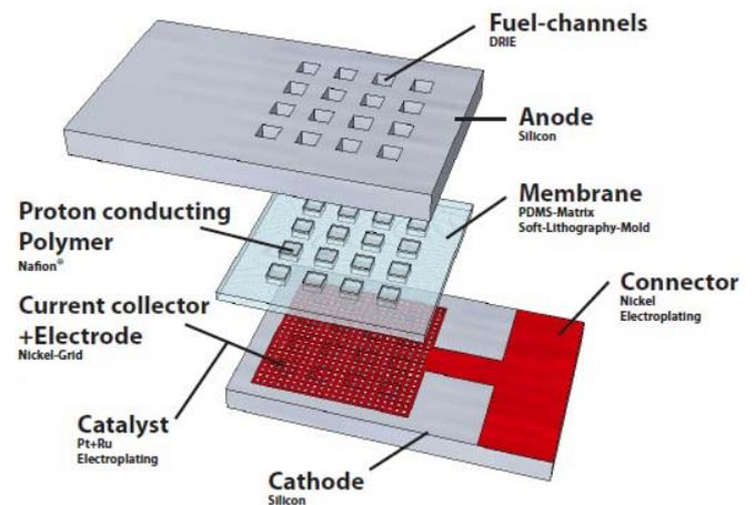
Fig. 1: Exploded view with detail and all parts of the proposed micro fuel cell identified.
