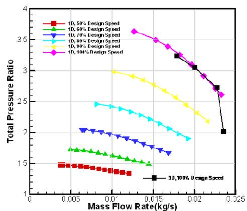
Figure 3 Total pressure ratio by the compressor
