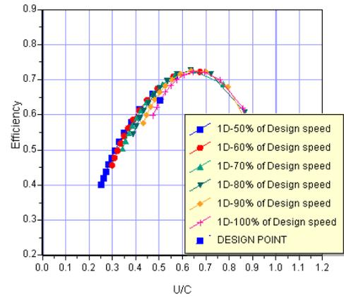
Figure 5 Blade speed vs efficiency by the turbine
