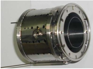
Figure 7 Annular combustor prototype
