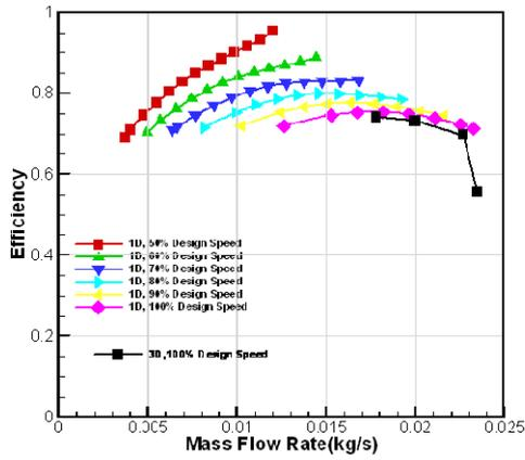
Figure 4 Efficiency of the compressor
