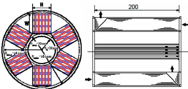
Figure 8 Plate stacked recuperator schematic
