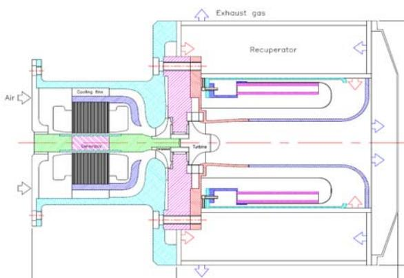
Figure 1 Schematics of the ultra-micro gas turbine
