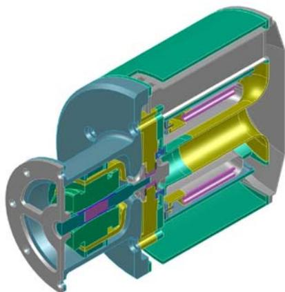
Figure 2 Three cutout of the ultra-micro gas turbine
