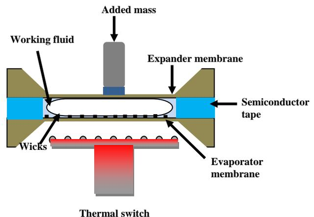
Fig.1. Schematic of micro heat engine.
