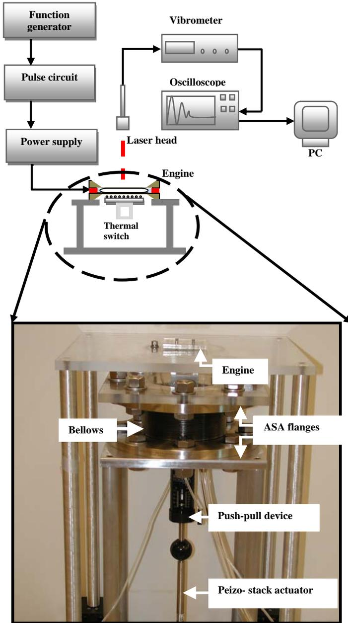
Fig. 2. Experimental setup apparatus.
