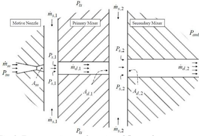
Fig. 1: Two-stage ejector schematic and flow paths
