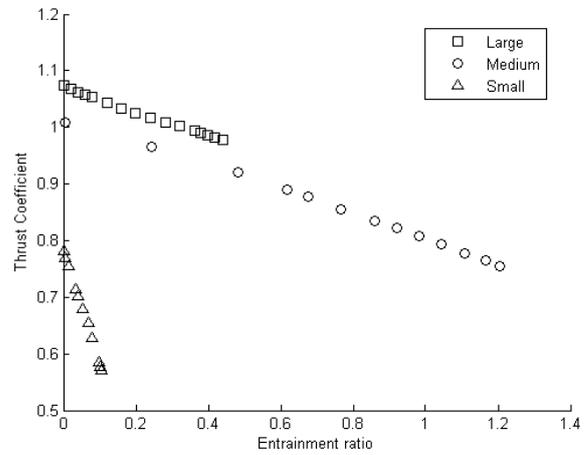
Fig. 4: Computed isentropic thrust coefficients vs. entrainment ratio
