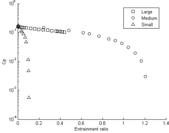
Fig. 3: Measured suction draft vs. entrainment ratio
