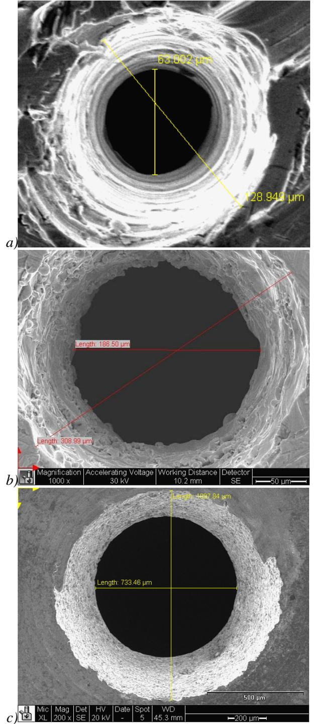
Fig. 2: Realized geometry for ejector motive nozzles. SEM images of a) 63  $\mu\text{m}$  nozzle, b) 187  $\mu\text{m}$  nozzle, c) 733  $\mu\text{m}$  nozzle.
