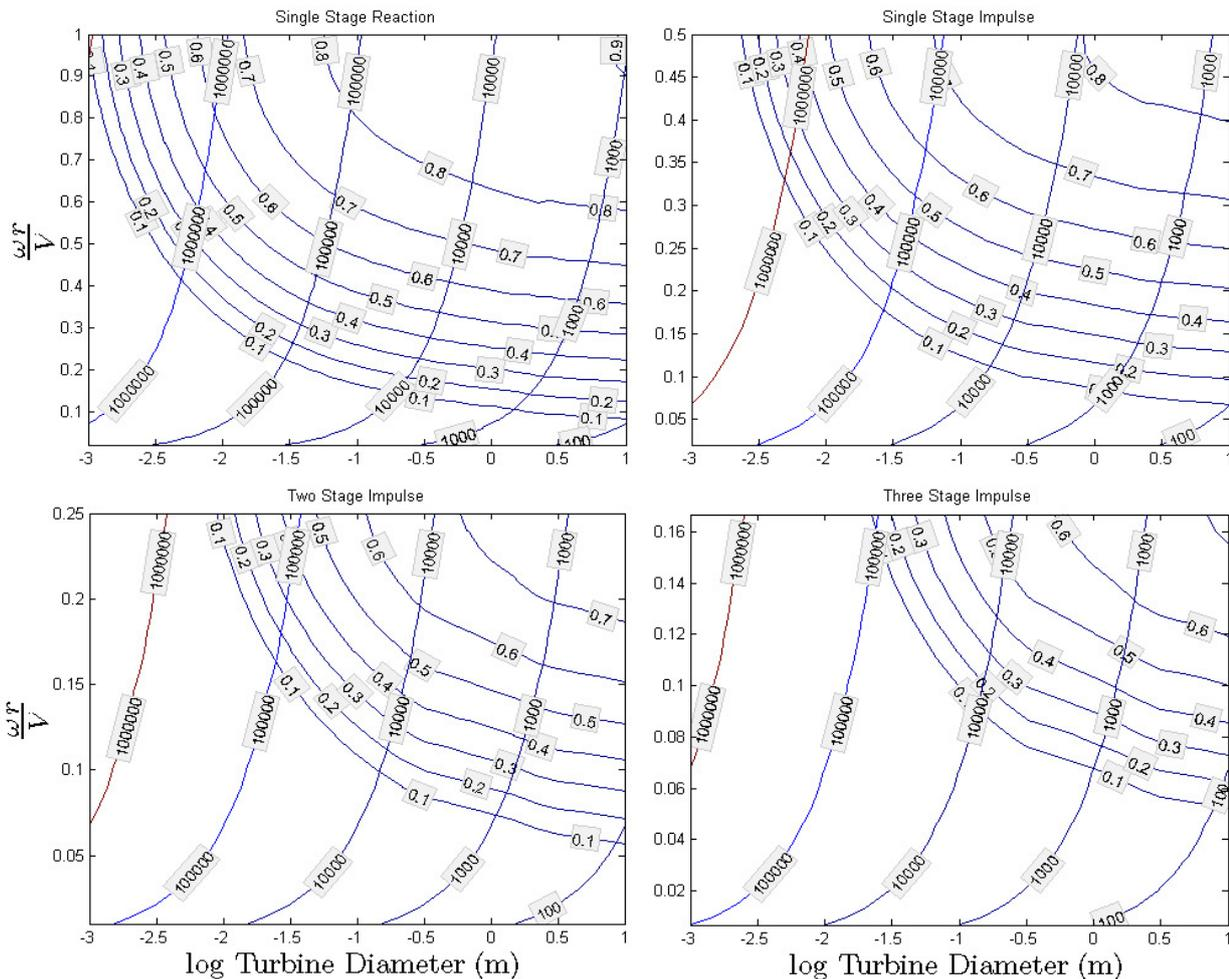
Fig. 6: Total-to-static efficiency of various turbines as a function of the velocity ratio, diameter, and RPM.
