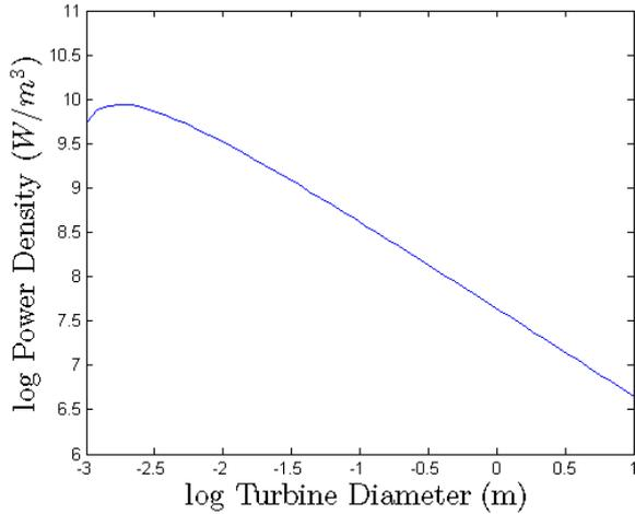
Fig 7. Power density of a single stage reaction turbine at optimal RPM as a function of diameter
