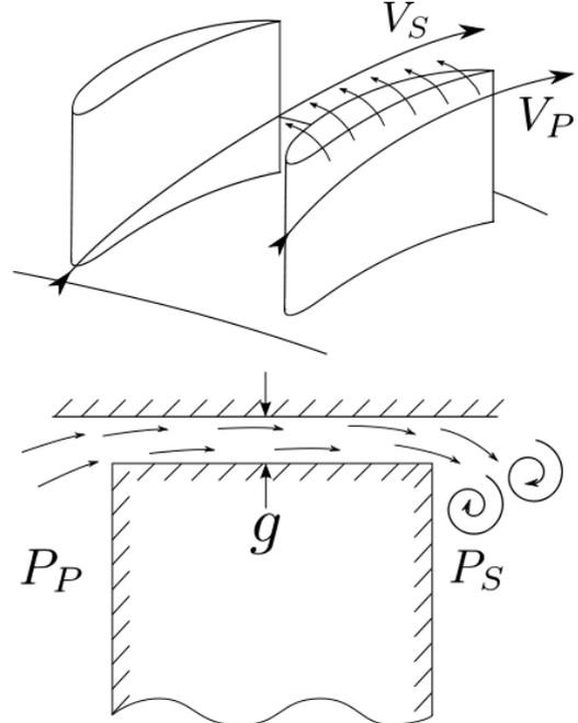
Fig. 5: Schematic of tip leakage.
