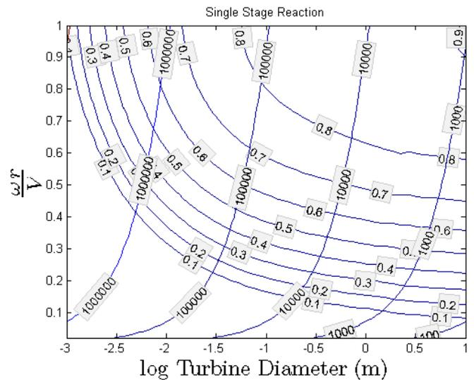
Fig. 1: Total-to-static efficiency of a single stage 50% reaction turbine as a function of the velocity ratio, diameter, and RPM.
