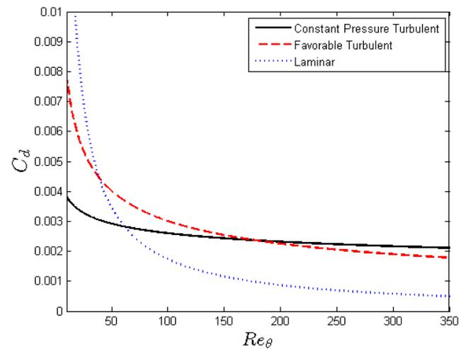
Fig. 3: Dissipation coefficient for various boundary layers.
