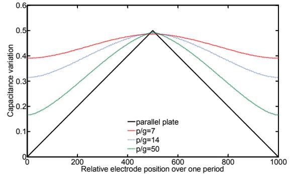
Fig. 2: The variation of  $C_1(x)$  for a range of  $p$  in  $x$ . The variation in  $C_2(x)$  would be identical only shifted by  $p/2$ .
