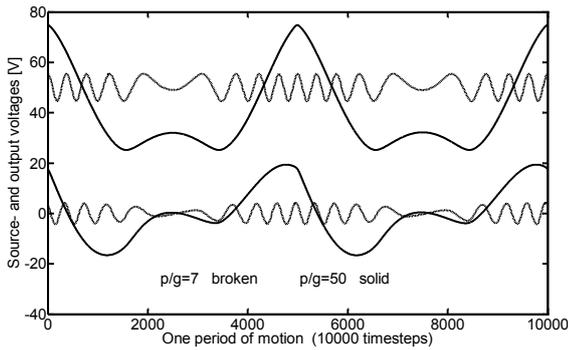
Fig. 3: Generated waveforms before and after RC filtering for two different  $p/g$  values.
