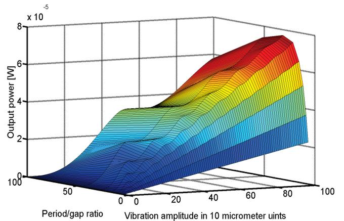
Fig. 6: The output power from a shuttle harvester as function of  $p/g$  and  $x_0$ .
