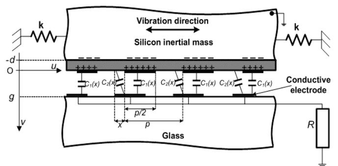
Fig. 1: The basic structure of the vibration scavenger. The capacitance values does not depend on  $d$  when  $d \ll p$ .
