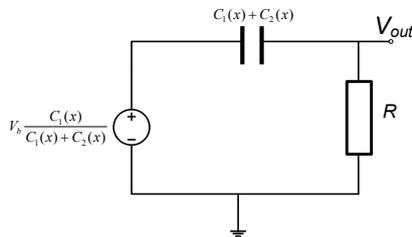
Fig.4: Electrical model of source and load.
