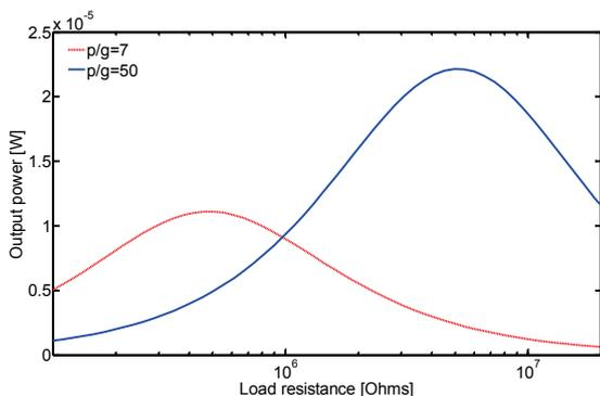
Fig. 5: Output power as function of the load resistance at two values of  $p/g$ .
