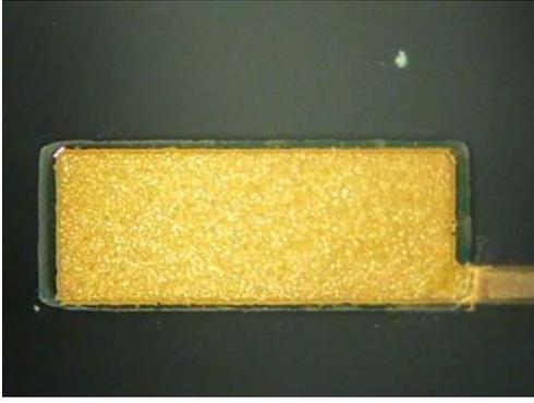
Fig. 5: the photograph of the fabricated PZT cantilever
