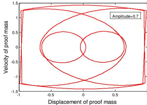
Fig. 7: Phase space trajectory in x-v plane for  $\hat{A}=0.70$ .
