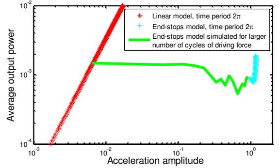
Fig. 4: Average output power versus acceleration amplitude.
