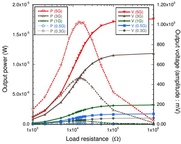
Fig. 6: Output voltage and generated power as a function of load resistance. The acceleration was varied from 3 m/s<sup>2</sup> to 50 m/s<sup>2</sup>.
