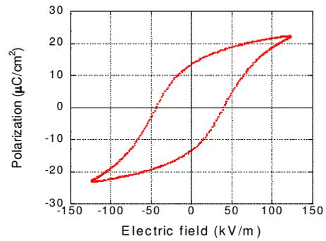
Fig. 4:  $P$ - $E$  hysteresis curve of the PZT film on Ti
