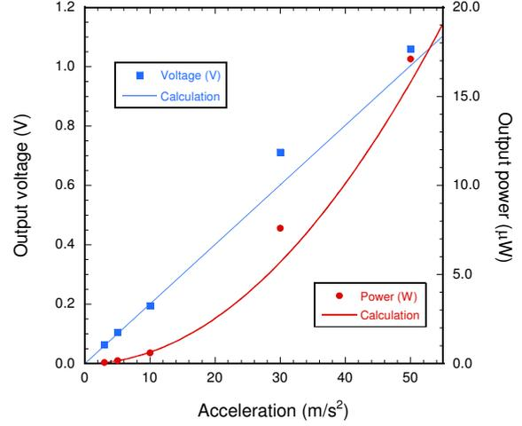
Fig. 7: Output voltage and generated power as a function of acceleration vibrated at the resonant frequency.
