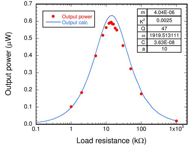
Fig. 8: Output power as a function of load resistance under the acceleration of 10 m/s<sup>2</sup>. The calculated curve corresponds with experimental values.
