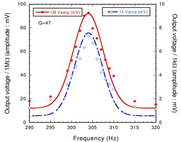
Fig. 5: Frequency response of output voltage under the acceleration of  $10 \text{ m/s}^2$  with the load resistance of  $1 \text{ M}\Omega$  and  $1 \text{ k}\Omega$ , respectively.
