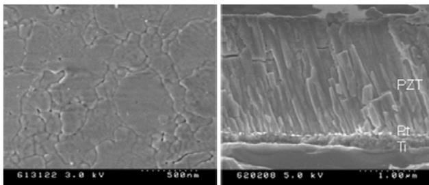
Fig. 3: Surface and cross-sectional SEM images of the PZT film grown on Pt-coated Ti substrate
