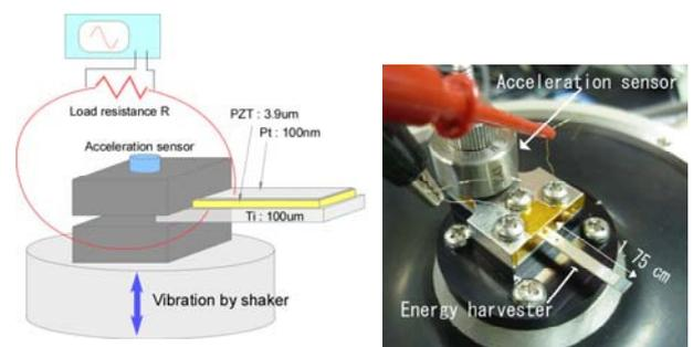
Fig. 1: A schematic and a photograph of piezoelectric energy harvester composed of PZT
