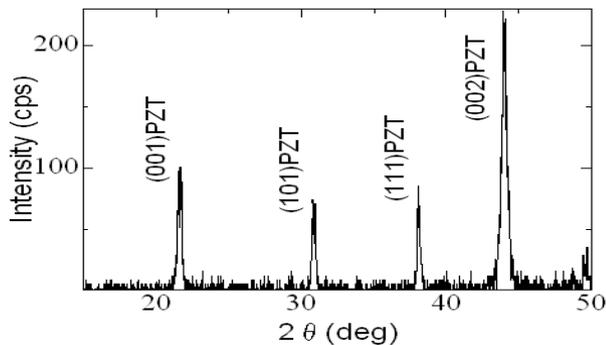
Fig. 2: XRD pattern of PZT films deposited on Ti
